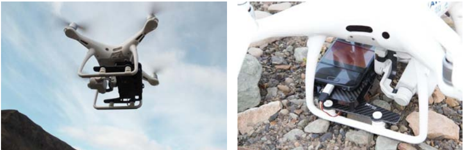
Fig. 23 – Customized DJI Phantom 4 Pro drone with a FLIR-ONE thermal camera + smartphone supplementary payload
