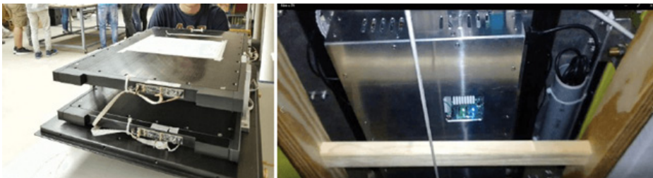
Fig. 16 – Cosmic ray detector after assembly at CERN (left) and installed onboard NANUQ (right)
