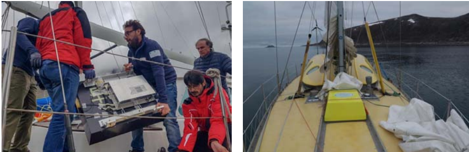
Fig. 30 – POLA-01 cosmic ray detector during installation on board (left) and ready to operate (right). The device is protected by an ad-hoc built fibreglass cover
