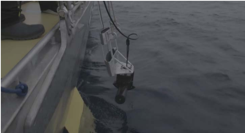
Fig. 63 – The multibeam sonar, attached to its aluminum bracket, is lowered into the water for installation onto the right daggerboard
