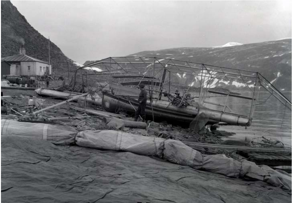
Fig. 108 – The wreck of Vaniman's gondola at Virgohamna after the failed 1909 flight. The bottom tank appears to be broken into parts which were to remain abandoned on site for over a century. Left in the background the «Wellman's Hut» is visible. An interesting detail is that the entire scene appears to be in an evident state of seasonal deglaciation, in a rather similar condition to that found by Polarquest2018
