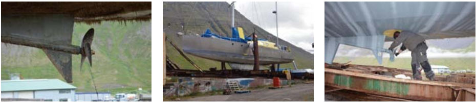
Fig. 29 – Keel cleaning and repainting; propeller change, July 20 th , Port of Ísafjörður Source: ph. by O. Pinazza and A. Margotti
