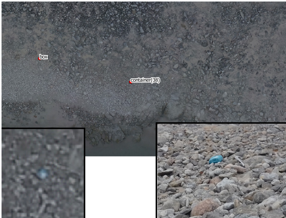
Fig. 118 – Documentation of artificial debris. Top: georeferenced ortophoto with points marking the position of debris. Left: a plastic fluid container as visible in the enlarged ortophoto. Right: the same container as observed during the ground truth session
