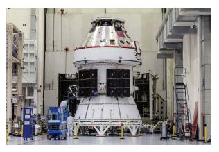
Figure 2: Orion crew vehicle with solar panels attached. (Courtesy of NASA)
