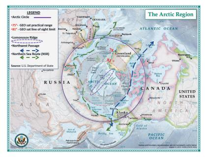
**Figure 1: The Arctic Region.** The smaller red circle (81°3') is the maximum latitude beyond which a geostationary satellite (GEO) is unable to provide coverage because it is below the local horizon. Operationally, a GEO satellite's limits are several degrees lower due to receiver noise from atmospheric refraction, frequency interference due to Earth's thermal emission, line-of-sight obstructions, and signal reflections with ground structures at approximately 75°.<sup>4</sup>
