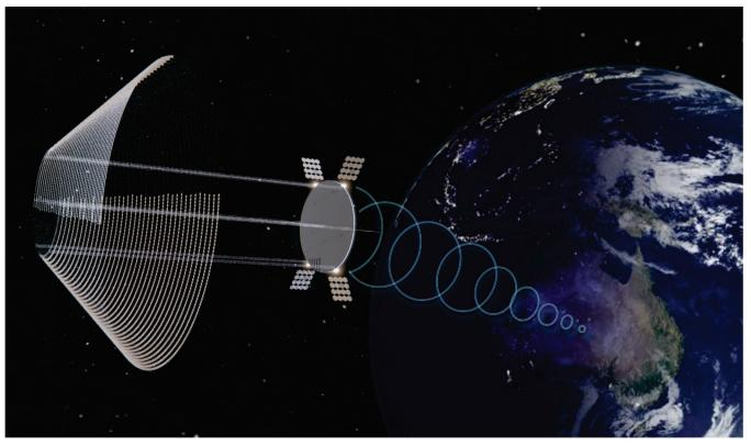
Figure 3: Highly modular SPS-ALPHA Mk-III space solar power system concept with light-weight structure and heliostat reflector array, transmitting power to Australia. (Image courtesy of John C. Mankins)
