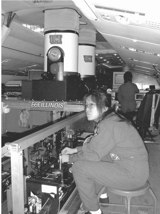
Fig. 4.6 Xinzhao Chu (foreground) and Weilin Pan operate the University of Illinois at Urbana two-beam Fe Boltzmann lidar installed in the NSF/Electra aircraft during the 1998 Leonid MAC mission. Photo courtesy: Chet Gardner, UIU.
