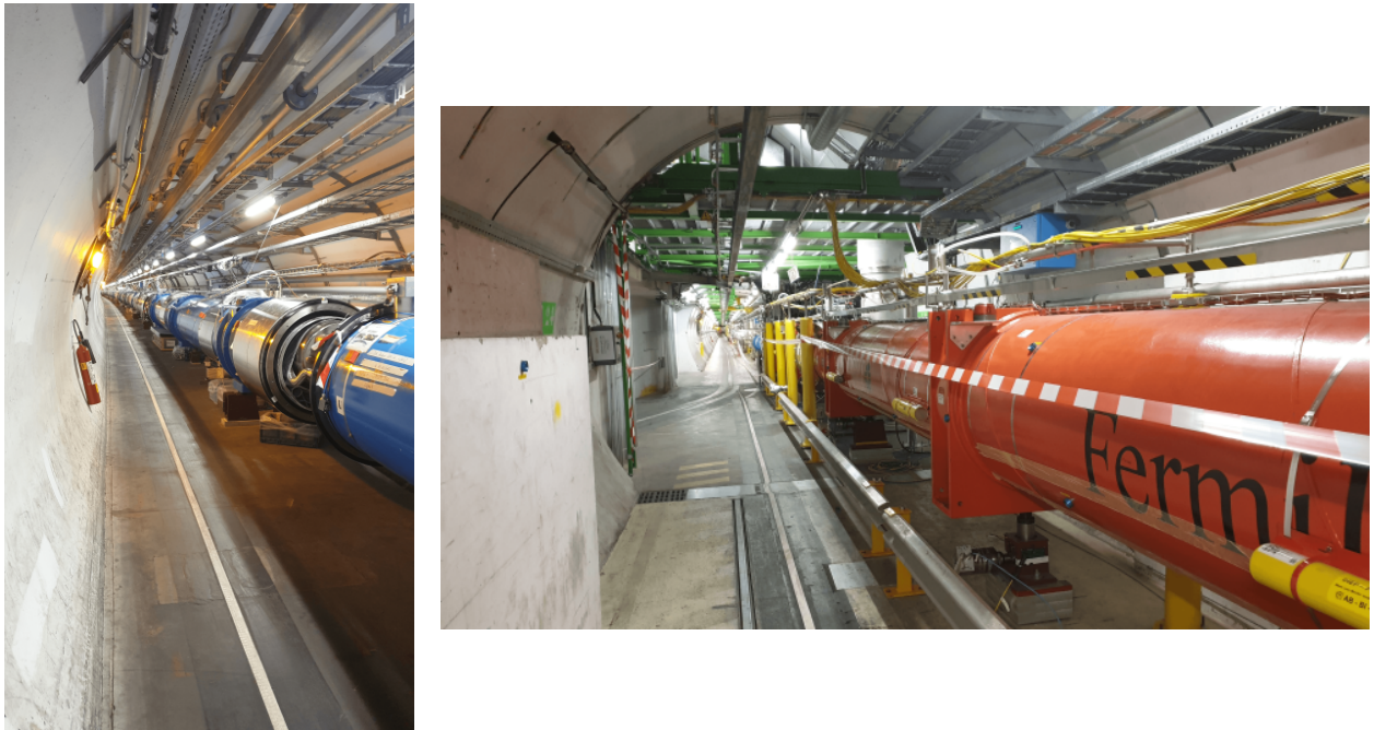
Figure 2.4: Left: An LHC quadrupole (chromium) between two dipoles (blue). Right: Inner triplet magnet (red) at A-side of the ALICE experiment for lowering the beam cross-section.
