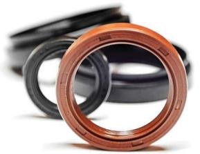
The primary factors determining O-ring material choices are chemical and temperature compatibility, sealing pressure, durometer, size, and cost. Additionally, electrical properties, dynamic resistance, tear resistance, and ozone resistance should be considered depending on the application.
