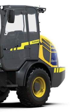
Komatsu machine, the traditional hydrostatic transmission that would normally be found on a wheel loader of this size was removed said Grabau. The servo motor used for traction is used instead to provide smooth forward and reverse operation as well as regenerative braking.
