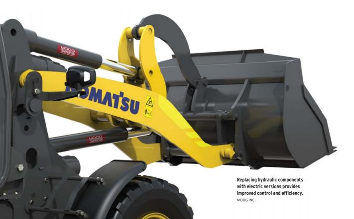
oog Inc. recently partnered with construction and mining machinery OEM Komatsu on the development of a fully electric compact wheel loader.
