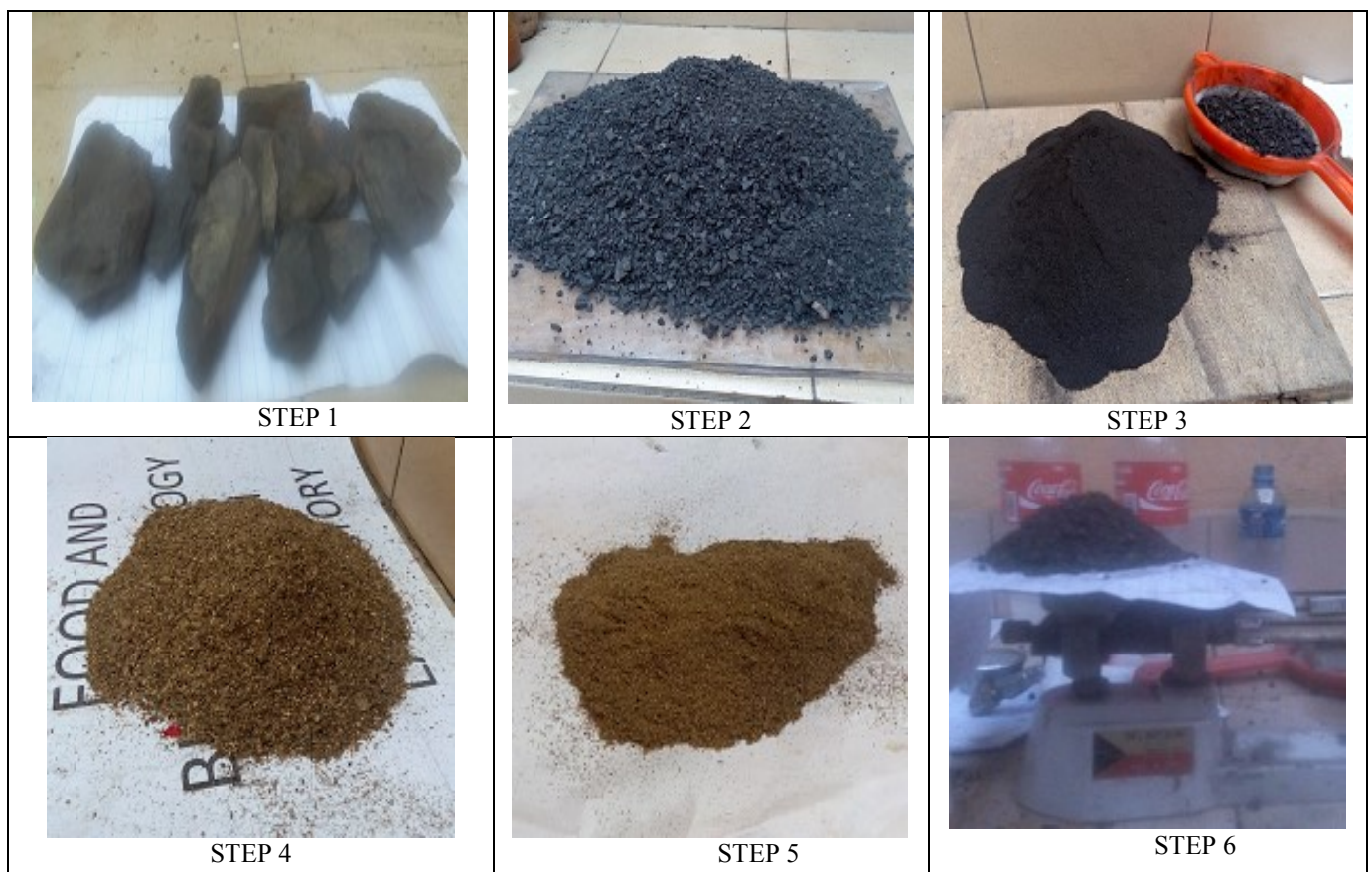
Figure 2. The basic flow process for bio-coal production
