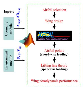
Figure 11. Scheme of the wing design process.
