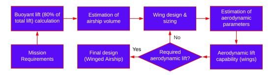
Figure 7. Sizing of envelope and wing for the given buoyant ratio (BR).
