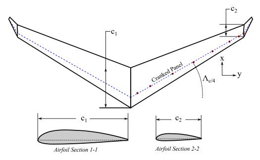
Figure 10. Cranked wing parameter definition.
