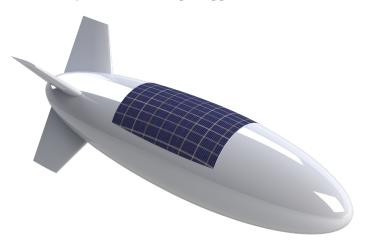
Figure 12. Airship with solar array.
