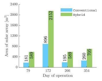
Figure 20. Area of solar array.
