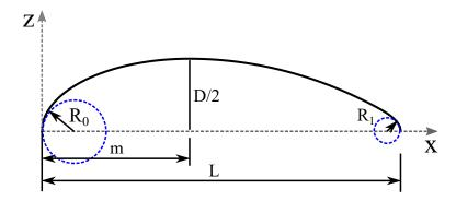
Figure 8. Design variables (geometric parameters) of the Gertler-58 Shape Generator.
