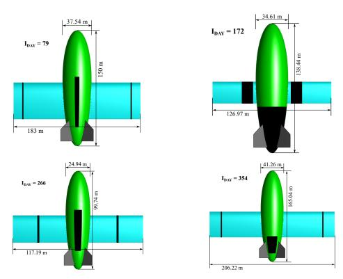
Figure 16. Optimum configurations—winged hybrid airship.
