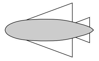
Figure 3. Airship with delta wings (Adapted from Ref. [31]).
