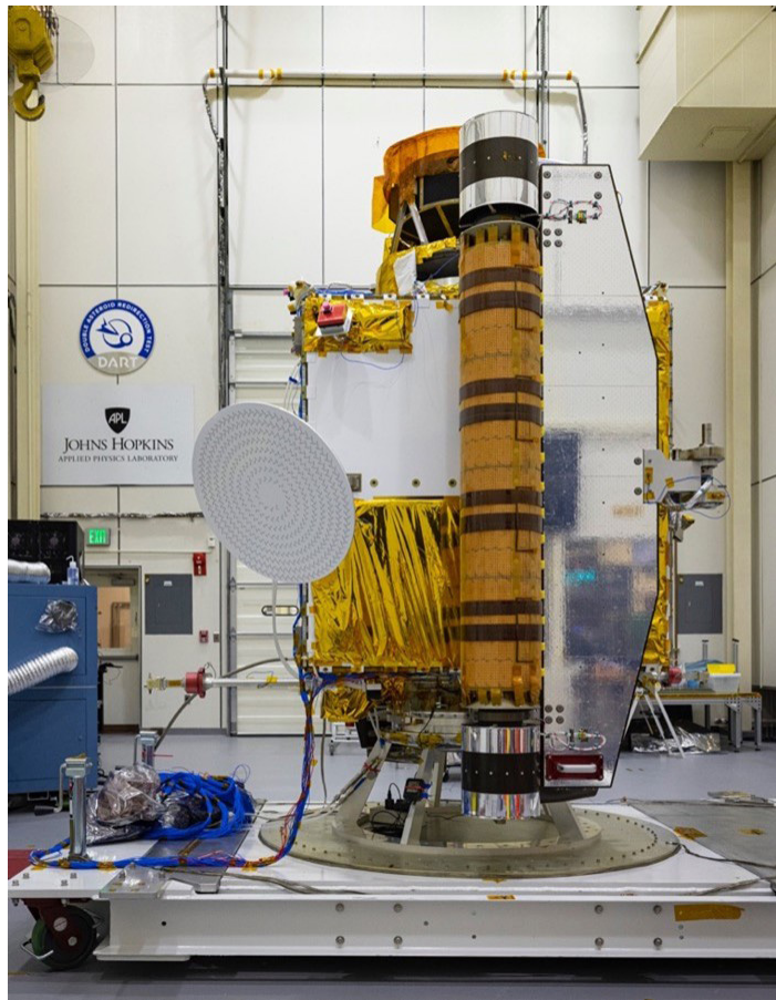
Figure 5. DART mechanical layout. The Radial Line Slot Array (RLSA), the solar array, and the radiator panel are clearly shown.
