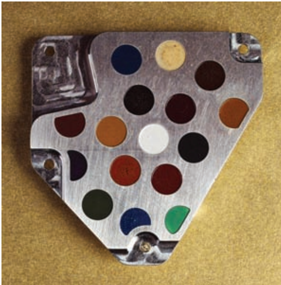
Plate 11 Damien Hirst, Beagle 2 Spot Painting , 2002, on gold background. Aluminum plate with indentations cut in the metal to accept colored spots in nine synthetic Mars iron oxides of different shades of yellow, red, orange, 8 × 8 cm, 26.5 grams. Known for his pricey zoological sculptures as well as his Spot Paintings , at times incorporated in earthly installations, this leading YBA (Young British Artist) practitioner hoped to install this Spot Painting with a useful chronometric function on Mars, as the visual art companion to a sound track to be played upon the Beagle's landing by the Brit indie band Blur. Although the Beagle crash-landed on a Martian plain, Damien Hirst's Spot Painting most likely remains partially intact.
