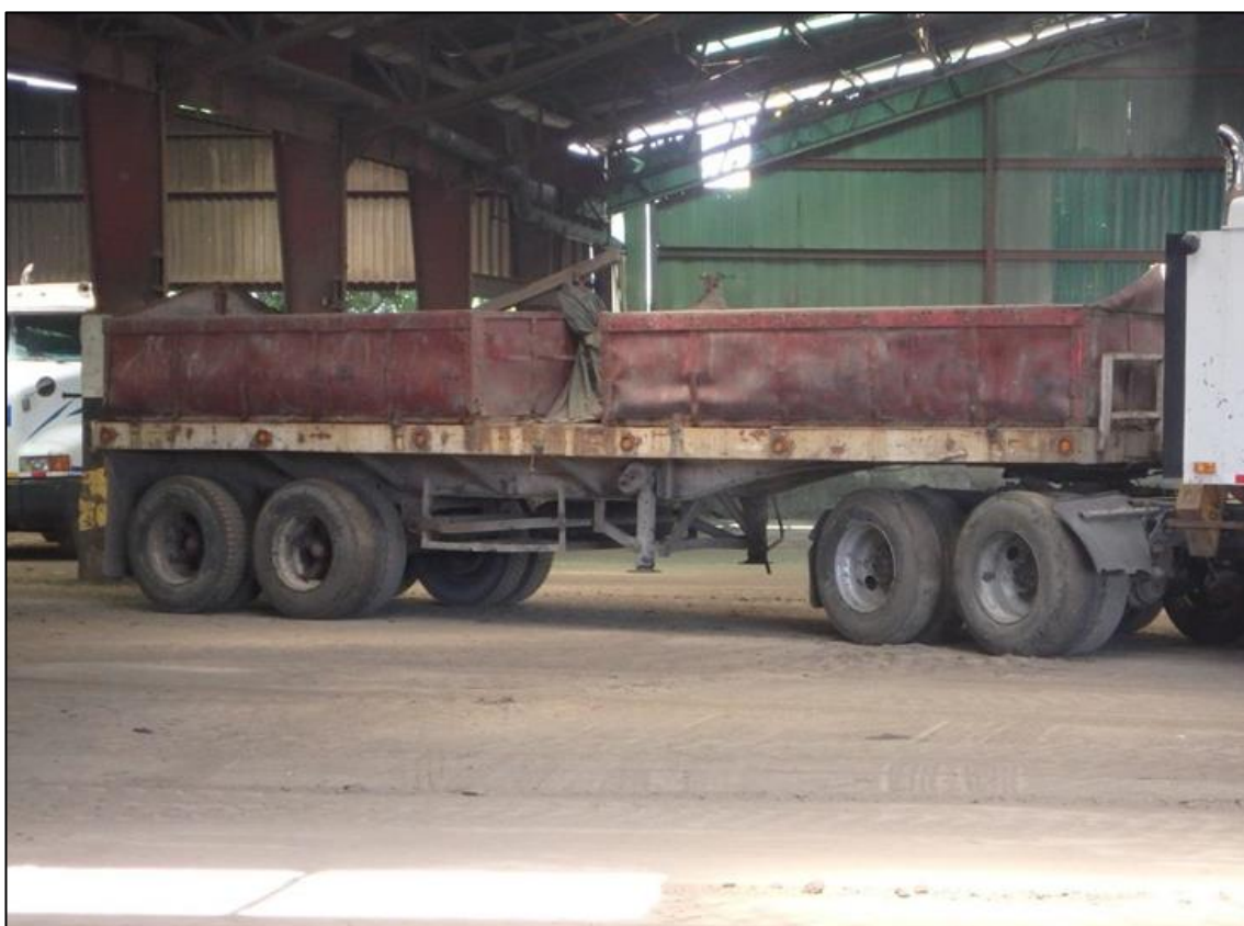
Figure 17.12 – Steel bins for concentrate transport
