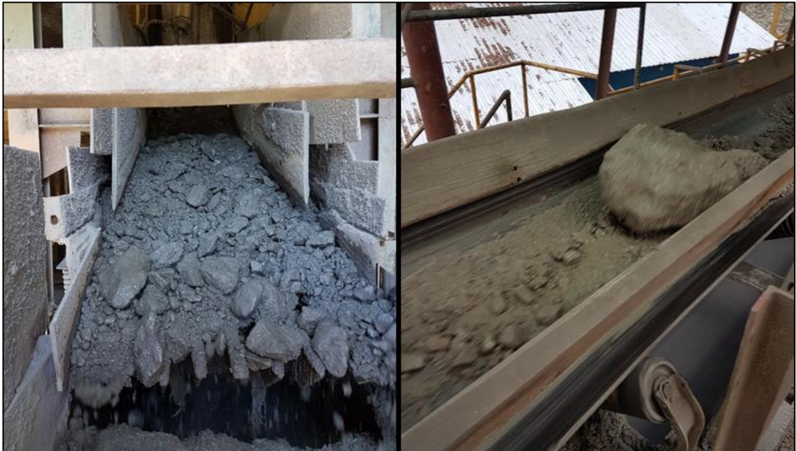
Figure 17.3 – (a) Jaw crusher grizzly feeder (b) Oversize rock (>0.5 m) on conveyor #2
