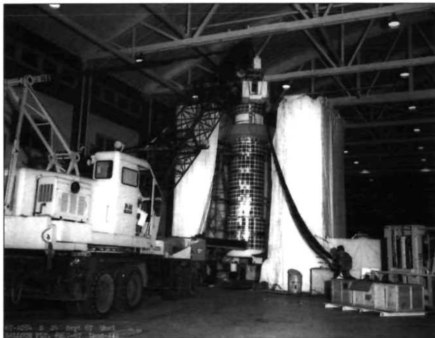
Pre-flight preparation of four-ton reconnaissance camera launched by a Skyhook balloon.
