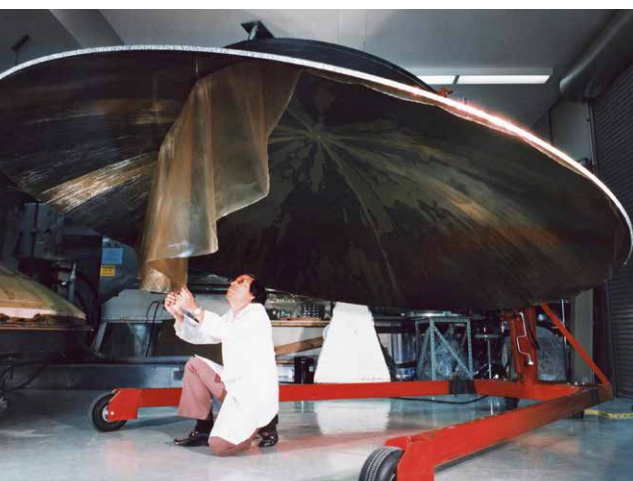
An engineer works on a Voyager spacecraft's high-gain antenna dish. A component necessary to transmitting data on the Voyager 2 spacecraft, the traveling-wave tube, is still functioning over 45 years later. Credit: NASA
