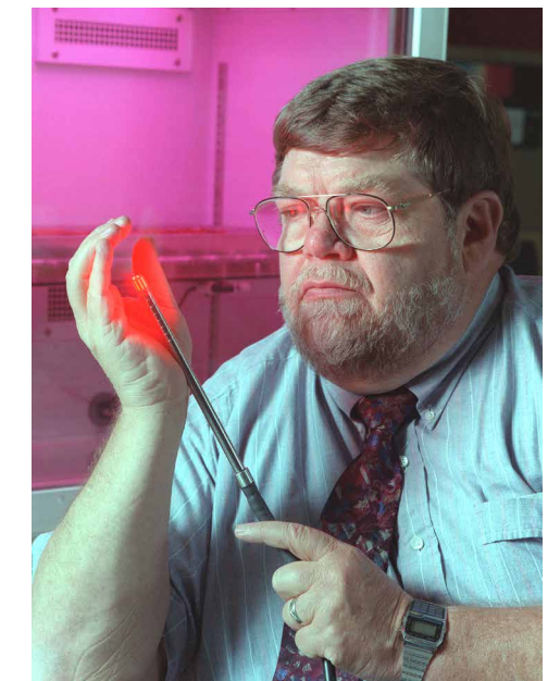
The late Quantum Devices founder Ron Ignatius holds what he referred to as a "photon cannon," capable of delivering a full watt of energy from LEDs alone. Marshall Space Flight Center partnered with Quantum Devices and others to explore the health benefits of certain light wavelengths and prove they could be effectively delivered by LEDs, giving rise to a light-therapy industry. Credit: NASA
