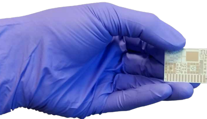
Utilizing NASA expertise, SBIR funding, and 3D printing, Ozark Integrated Circuits created a single-board computer module that withstands extreme heat and doesn't require a bulky cooling system. This makes it possible to embed sensors and electronics in geothermal drilling equipment, jet engines, and other Earth applications. Credit: Ozark Integrated Circuits Inc.
