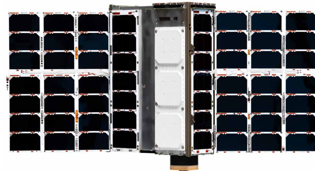
Spire Global currently has the most radio occultation satellites in orbit, having outfitted 40 of its Low Earth Multi-Use Receiver (LEMUR) satellites with radio receivers capable of the technique. Credit: Spire Global Inc.
