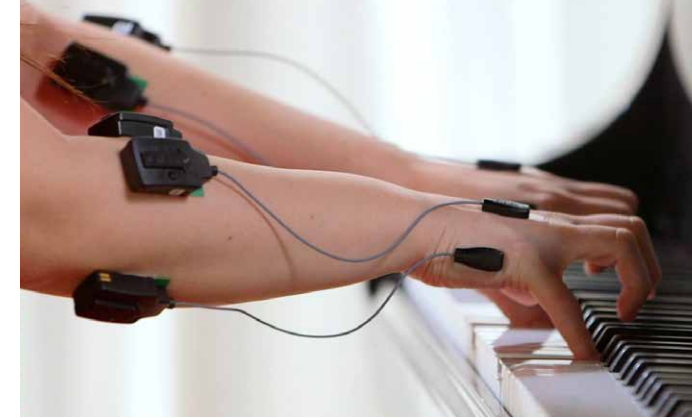
Trigno Mini sensors are applied to the forearm and hand muscles of professional pianist Rui Urayama to gain understanding of fine motor control strategies. Credit: Delsys Inc.
