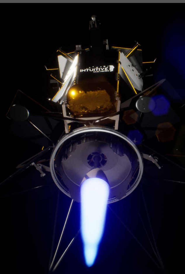
Intuitive Machines' Nova-C lander, shown in this artist's rendering, uses a liquid methane propulsion system, one of a handful of similarities between this commercial lunar lander and the experimental Morpheus lander that several of the company's engineers helped build when they worked for NASA. Credit: Intuitive Machines LLC
