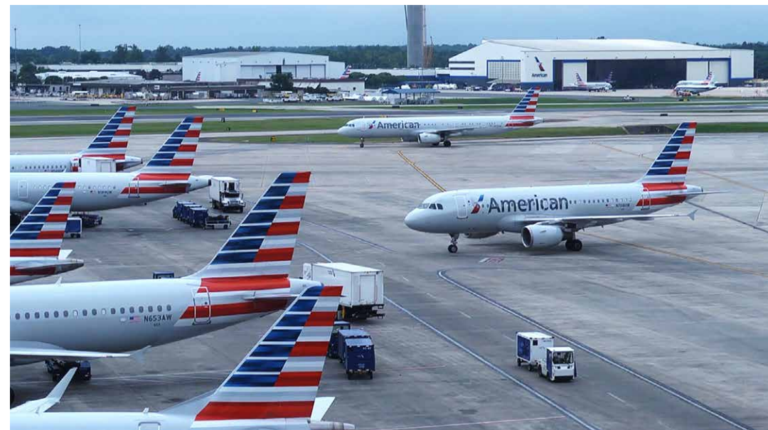
Holding airplanes at the gate until just before takeoff allows them to run on power supplied by the airport. American Airlines saved hundreds of thousands of gallons of fuel, as well as maintenance costs and thousands of tons of harmful emissions by only running engines when arriving at and leaving the gate. Credit: NASA
