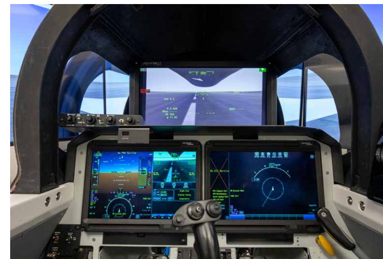
With no forward-facing windows, the pilot will rely on a digital display like the one in this rendering of the X-59 cockpit. A custom external vision system includes two cameras that will act as the pilot's eyes. To meet NASA's specifications, the company Eon Instrumentation had to create a DisplayPort switcher/converter capable of instantaneously switching between ultra-high-definition video feeds. With an overlay of important flight information, the pilot will have all the essential information on one display. Credit: Lockheed Martin Corporation
