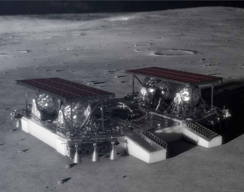
Landing on a lunar surface is risky, but making the craft as light as possible helps. The mid-sized lander concept in this illustration, which would deliver a rover to the polar regions of the Moon, could benefit from a lightweight carbon composite tank developed by Gloyer-Taylor Laboratories. Credit: NASA
