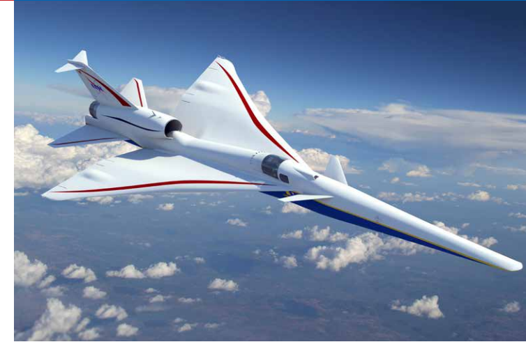
The NASA Quiet SuperSonic Technology Low-Boom Flight Demonstrator, also called the X-59, is designed to prove it's possible to take the loud boom out of supersonic flight. The aircraft design changes the structure of the sound wave, making it more like a thump. This is one step toward removing the overland flight ban for planes traveling faster than the speed of sound. Credit: Lockheed Martin Corporation
