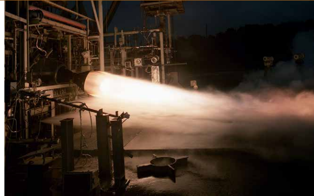
A Fastrac engine undergoes testing at Marshall Space Flight Center. The turbopump used in this design was manufactured by Barber-Nichols, which went on to produce similar designs for companies such as SpaceX. Credit: NASA
