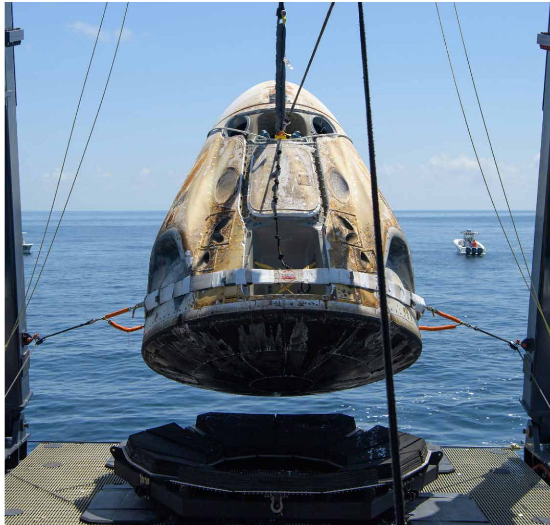
The scorched SpaceX Crew Dragon Endeavour capsule is lifted out of the Gulf of Mexico after safely carrying NASA astronauts Robert Behnken and Douglas Hurley from the International Space Station back through Earth’s atmosphere in 2020. To ensure the capsule’s safety and durability under stresses like liftoff and atmospheric reentry, SpaceX engineers used NASGRO software to predict the behavior of any possible cracks or damage to the structure. NASA invented NASGRO to evaluate the world’s first reusable spacecraft, the space shuttle. Credit: NASA
