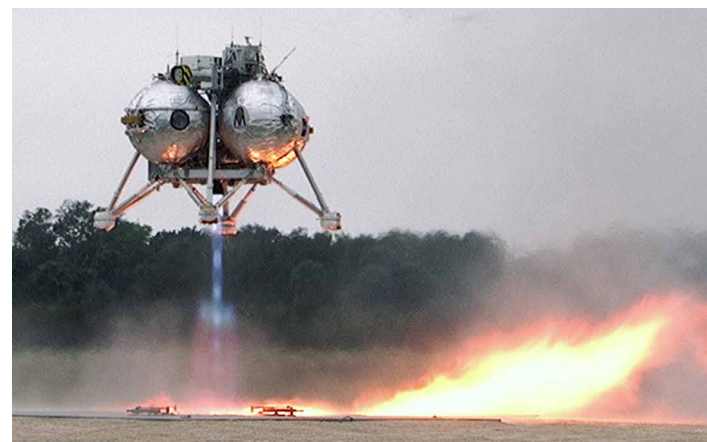
Between 2010 and 2014, Project Morpheus at Johnson Space Center developed a vertical-landing test vehicle to try out landing navigation technology and nontoxic liquid methane propulsion. Now several of the engineers who worked on the project have applied some of that technical knowledge to one of the first commercial lunar landers, Intuitive Machines' Nova-C lander. Credit: NASA
