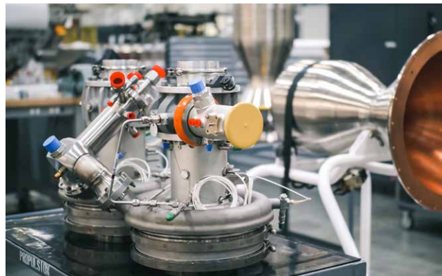
These turbopumps are used in the NewtonThree engine from the first stage of Virgin Orbit's LauncherOne rocket. Produced by Barber-Nichols and similar in design and principle to pumps originally made for NASA, the pumps move liquid fuel into a rocket engine that ignites after being dropped from an airplane. Credit: Virgin Orbit
