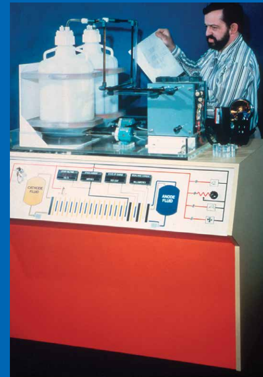
In developing its flow battery, ESS drew from groundbreaking research and development conducted by the space agency more than 40 years ago. Pictured here is a 200-watt demonstration unit of the flow battery NASA built in the 1970s and 1980s. Credit: NASA
