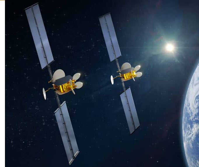
Northrop Grumman's first major customer for its new, NASA-based Compact Telescoping Array (CTA) solar panel design is Airbus, which is using the panels on its new OneSat communication satellites, shown in this artist's rendering. Credit: Airbus Defence and Space Ltd.
