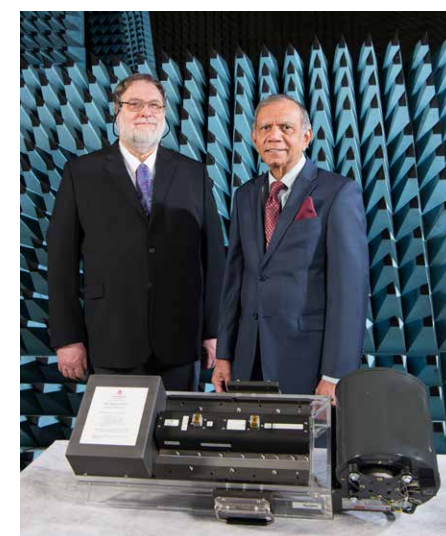
NASA electronics engineers Dale Force and Rainee Simons with an L3 (now Stellant) traveling-wave tube amplifier (TWT). Today, Stellant is the only company making space-rated TWTAs and has several private sector customers in addition to NASA. Credit: NASA
