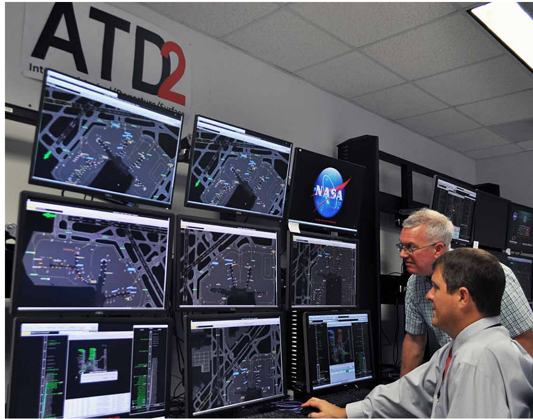
The focus of Airspace Technology Demonstration 2 was IADS, a software that coordinates flight schedules between the ramp, tower, terminal, and center control facilities. This visual representation of data helps minimize delays on the ground. Credit: NASA
