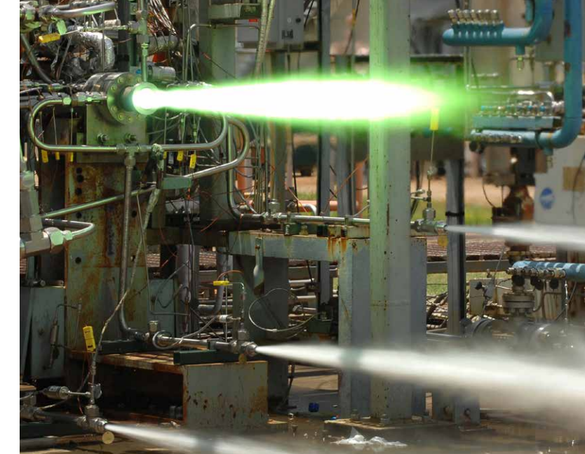
This hot-fire test of a 3D-printed rocket engine injector was successful, with post-test inspections revealing the injector remained in such excellent condition and performed so well that it went into acoustic tests. Now engineers can use DC-AM to design, build, and test parts like this in a virtual environment created by Sentient Science. Credit: NASA
