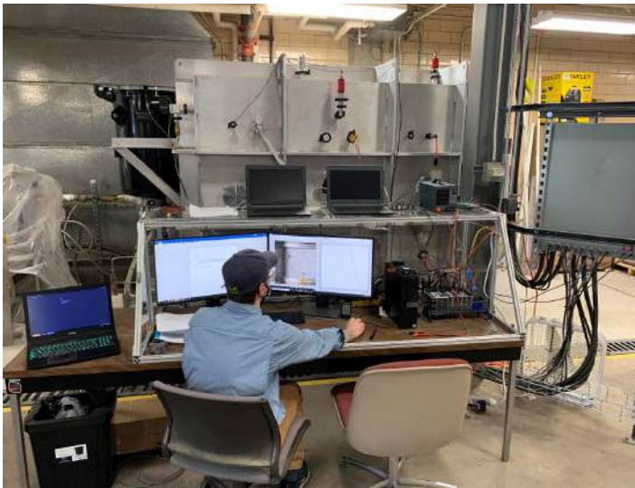
Figure 7: Testing with MTU-LHT-1A lunar simulant inside the DTVC.
