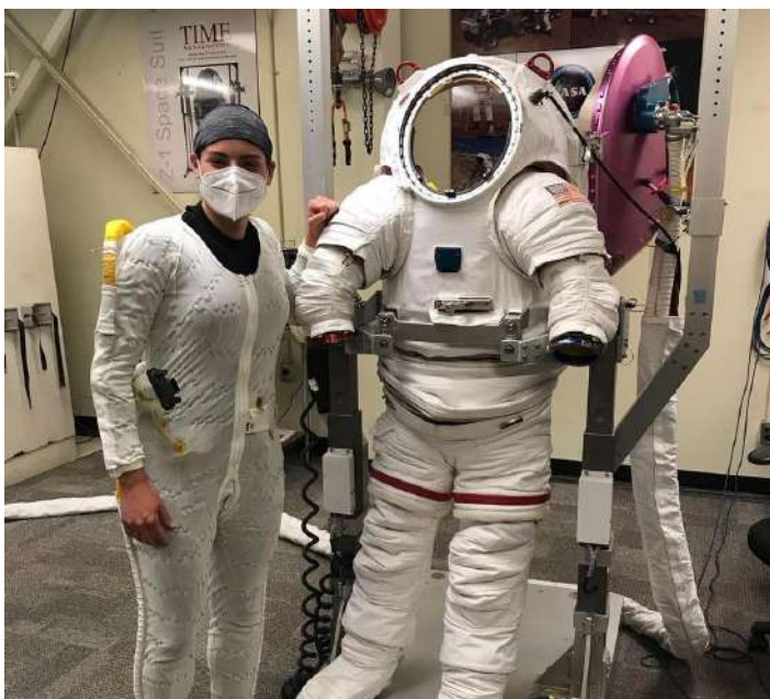
Figure 6: Dr. Dunn, REVEALS team testing the functionality of the cooling garment design at Johnson Space Center.
