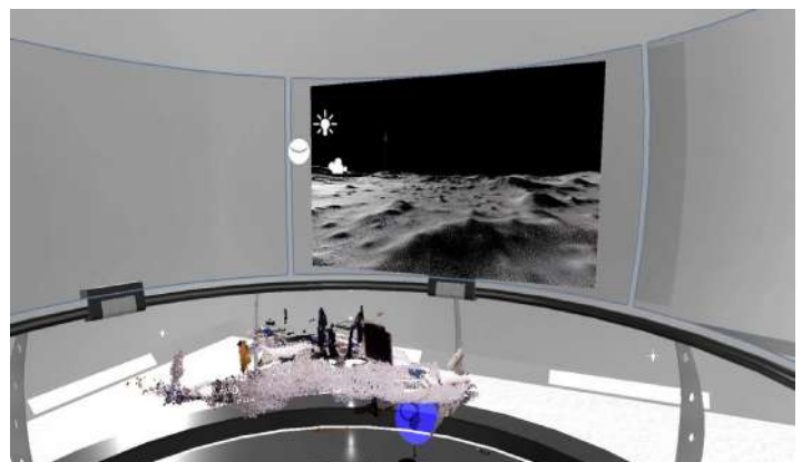
Fig. 5 - The NESS hybrid augmented virtuality interface design unifies concepts from both cyber-physical and virtual control room interfaces by providing mobile space robot operators with egocentric (live 3D video stream) and exocentric (3D dense point cloud environmental constructions) perspectives to enhance telepresence and situational awareness.
