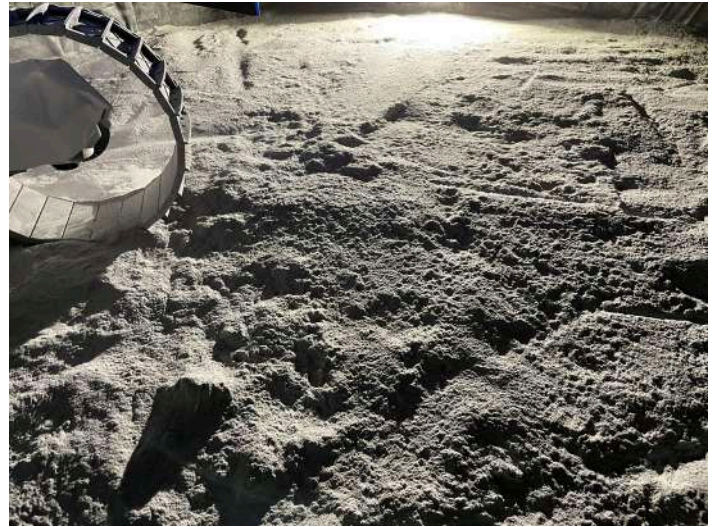
A wheel from the mockup for the VIPER mission to verify hazard camera beam pattern, placement and visual results from simulations
