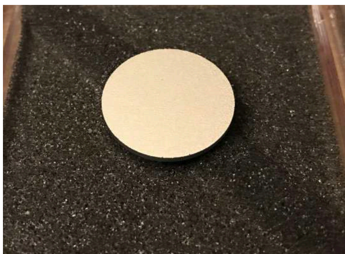
Figure 1. A sample glass disk coated in platinum, an excellent calibration standard for UV-visible wavelength measurements.
