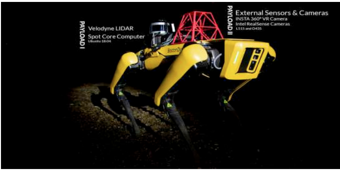
Figure 1A. Boston Dynamics Spot robot equipped with multiple payload elements on RESOURCE 2021 deployment.
