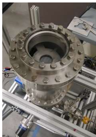
Figure 3: Experiments are underway examining the feasibility of extracting volatiles from the regolith using solar power. The principle of operation is shown in the top left figure. The simulator was calibrated to a thermal radiative flux of 35 kW/m 2 . Figure below documents the temperature of the apparatus. The low flux is necessary to avoid damaging the quartz window.
