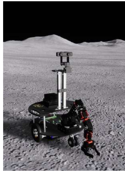
Fig. 7 The digital twin of the NESS Armstrong rover and mechanical arm on the simulated lunar landscape within NESS's VR construct.
