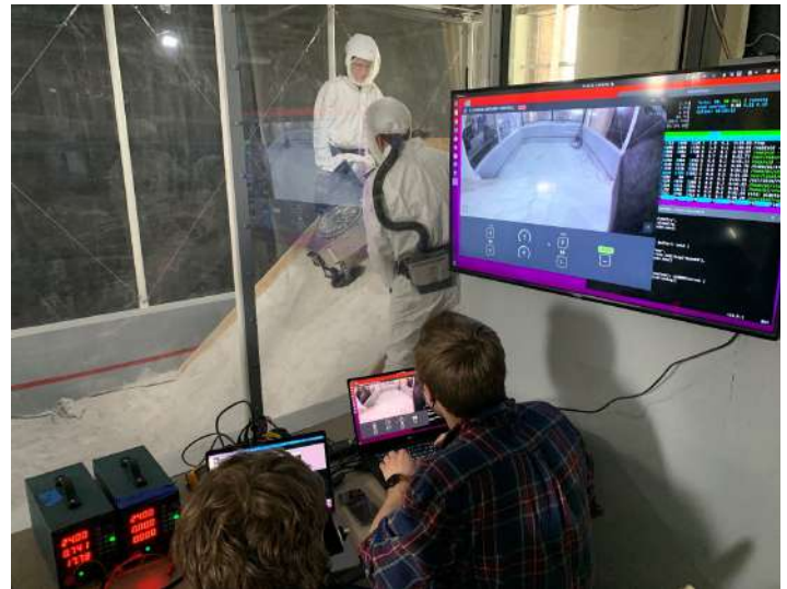
Figure 8: Testing T-REX on the first batch of in-house created MTU-LHT-1A lunar simulant.
