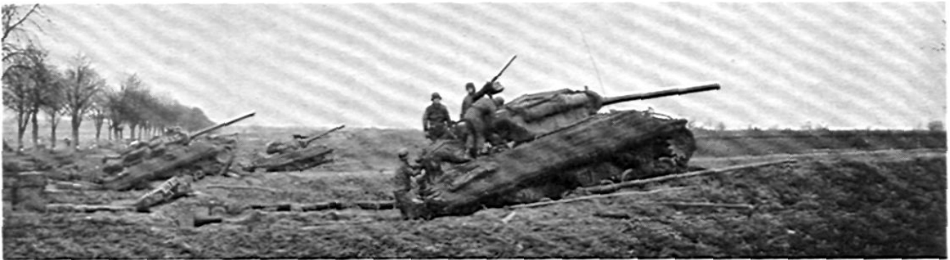
For long range fire across the Roer River the tank destroyers of the 2nd Armored Division, Ninth Army, had to dig ramps to gain extra elevation.
