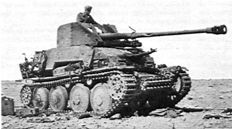
By the time of our North African campaigns the Germans had mounted Russian 76.2-mm antitank guns on the Czech (Skoda) T.N.H.P. light (10-ton) tank chassis.
