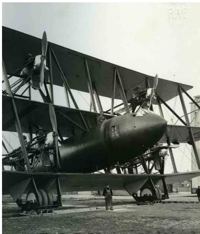
Figure 28. Close-up of the Tabor showing the six Napier Lion engines and the problematic undercarriage. Note the limited ground clearance of the cross-beams at front.
