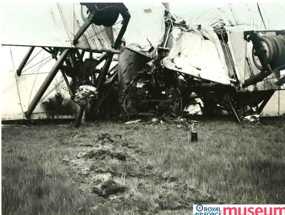
Figure 43. Close-up showing the final path of the Tabor and complete destruction of the forward section, up to the mating ring. RAF Museum, PC72/100/231
