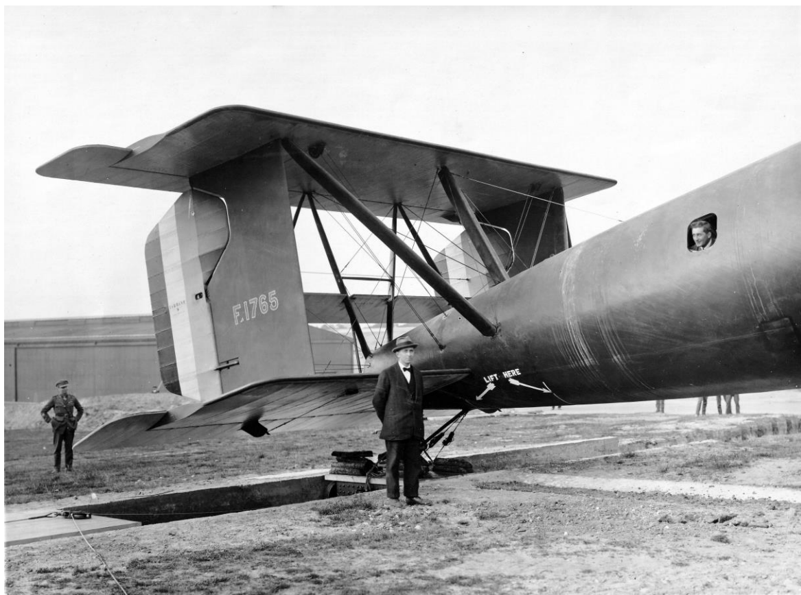
Figure 26. The Tabor's massive tail assembly comprising two rudders and three elevators. Wilson stands at the rear, Rawlings before the tail and the test pilot Dunn inside the fuselage (the position Wilson took on the test flight.)
