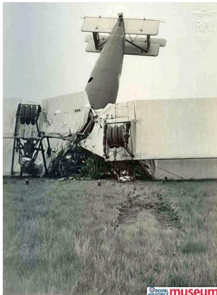
Figure 44. View of the Tabor's undercarriage showing distortion of both front I-beams as they impacted and then ploughed the ground
