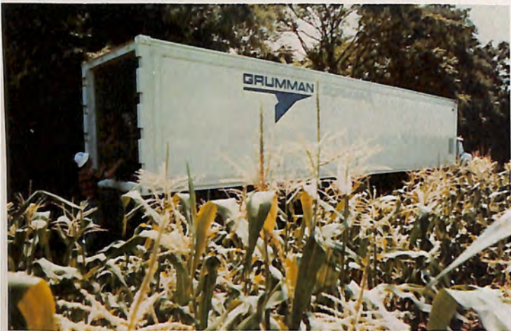
Grumman's Dormavac, a spinoff from the company's work on space environmental control, provides a commodity-preserving environment for long-term protection of perishables without freezing.
