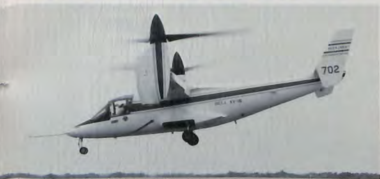
Tilt-rotor Plane. Shown on its first hover flight earlier this year, Bell Helicopter Textron's XV-15 combines the best features of helicopters and fixed-wing aircraft. Its rotors operate in the horizontal plane for helicopter-like take-off, then tilt forward to become propellers for fast forward flight.
