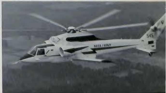
Flying Wind Tunnel. The NASA/Army/Sikorsky Rotor Systems Research Aircraft is an airborne laboratory for testing a variety of advanced rotor systems. It can be flown as a conventional helicopter or, as shown above, as a compound helicopter, a winged rotorcraft which has the higher cruise speed of an airplane although it retains the helicopter's vertical flight characteristics.
