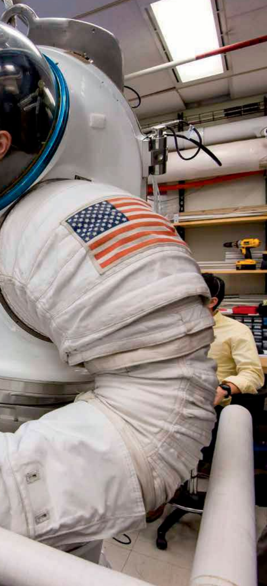
◀ A NASA spacesuit engineer wears a prototype spacesuit during a test of the Portable Life Support System 2.0. NASA
