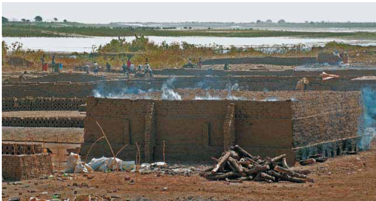
Brick kilns on the banks of the Blue Nile, in El Gezira state. The brick-making industry is a major market for fuelwood
