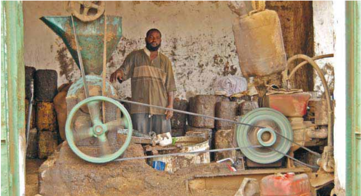
A small sesame seed oil pressing plant in Port Sudan. Food processing represents a significant part of the light industry sector in Sudan
