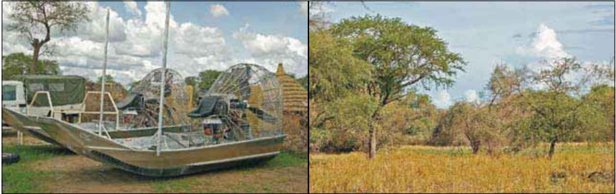
Airboats used for seismic surveying access in the swamps and floodplains of Jonglei state, reducing the need for access roads in the first stages of oil exploration
