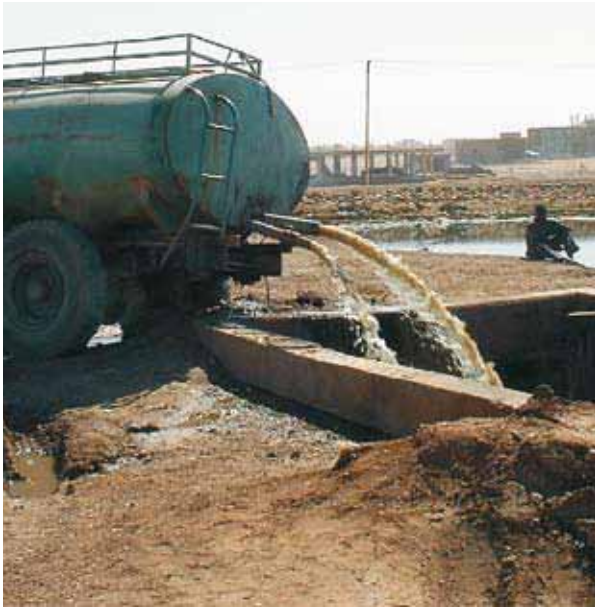
The majority of the urban population of Sudan relies on basic latrines or septic tanks that are emptied by truck. In this case, the load is transferred to the Khartoum sewage works
