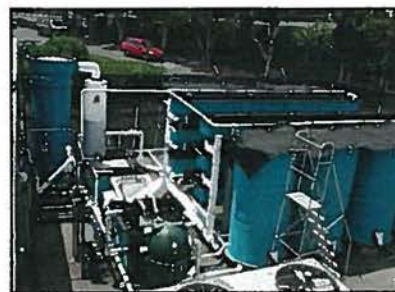
Figure I-2. Recirculating flatfish larval and juvenile system.
