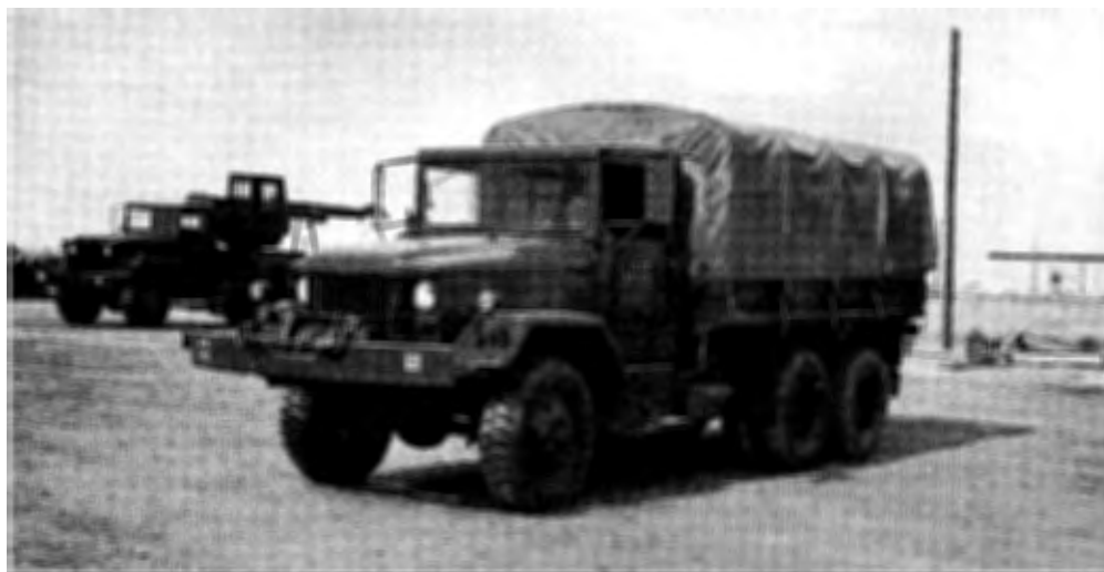
Fig. 31. An M-35 2 ½-ton cargo truck, commonly referred to as a “six-by-six,” were used by the Holloman Balloon Branch to launch and recover anthropomorphic dummies and suspension racks at numerous locations throughout New Mexico. (U.S. Air Force photo)
