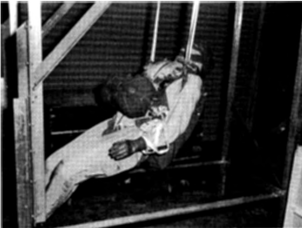
Fig. 74. “They looked like they had some sort of bandages on ‘em...over his... arm... around his midsection and partially over his shoulder”—witness description of tape and nylon webbing used to prevent arms and legs from flailing, and parachute harness that had chest and shoulder straps. Tape was also used to secure the removable back plate of the head (also see figs. 29, 30, 73,75). (U.S. Air Force photo)
