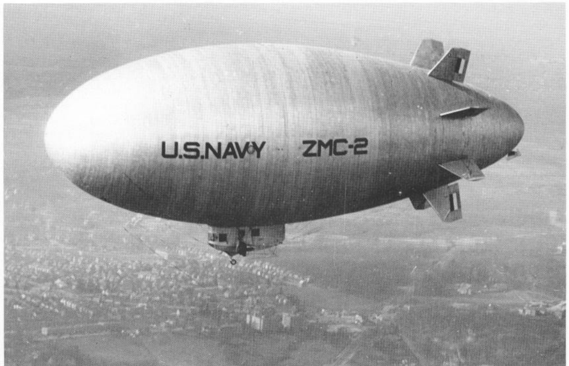
The ZMC-2, shown here on a flight over Washington, D.C., was the only metal-clad airship.
