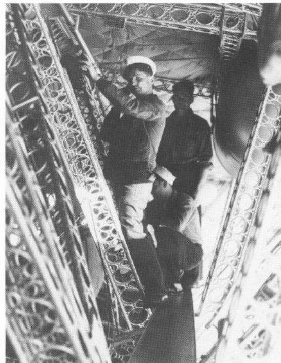
Below left, Macon approaching the mooring mast at NAS Sunnyvale. Below, an interior view of the port catwalk on Macon.
