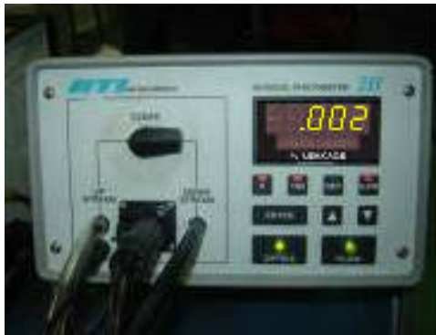
Fig. 4. Resultado correcto: no fuga Correct result: there isn't Leak
