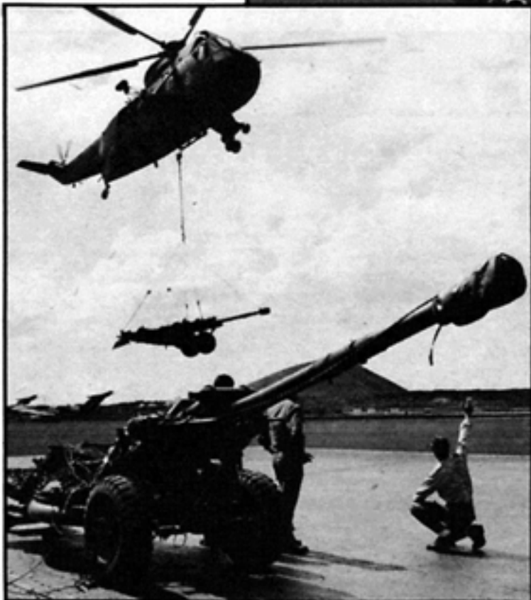
BELOW: The 105mm light guns of 29 Commando Royal Artillery are lifted by Sea King helicopters of 846 Squadron. On the airstrip apron in the background are two Victor tanker aircraft.
