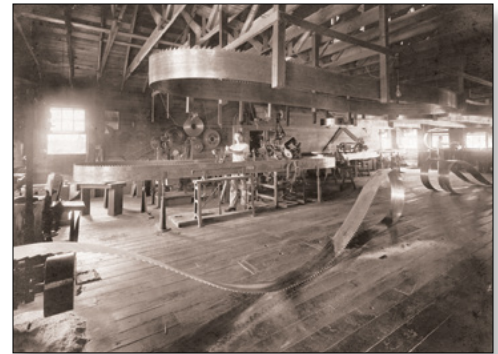
Typically, on the third floor of the mill was the area for the saw filer to use for sharpening the band saws. The filer was one of the highest paid employees of the mill. His effectiveness was essential in maintaining the productivity of the sawmill. (Photo from The History Center’s online collections [www.thehistorycenteronline.com])
