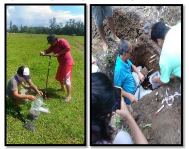
Figure 2.1 Auger Boring and Pit Boring
