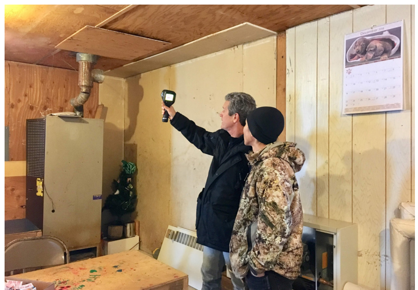
The energy auditor and Atmautluak's tribal administrator use a thermal camera to examine the building envelope of the gaming office.
