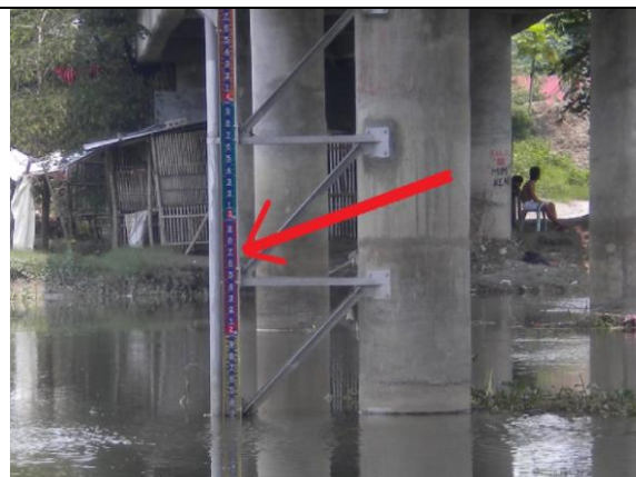
River crested at almost 2.72 meters (flood marks) at the Mexico RR and WL station. Peak was attained at around 0800H of June 25.
