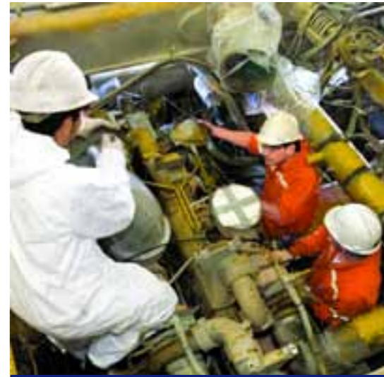
Matías Acosta, Daniel Palacios and Manuel Caracho repairing a 793 haul truck engine.
