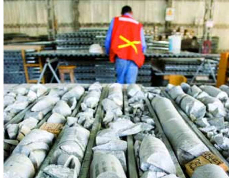
Drill cores corresponding to the exploration programme of new reserves in the deposit.
