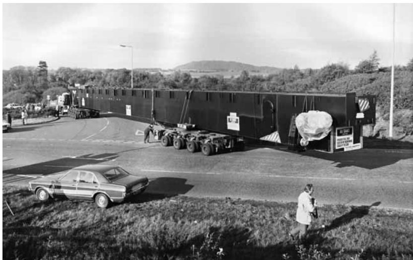
1981: Firmly strapped to its transport, this girder for a coking crane at Immingham Docks was the longest load ever to be carried by road at that time (© courtesy of Dawley History Group)
