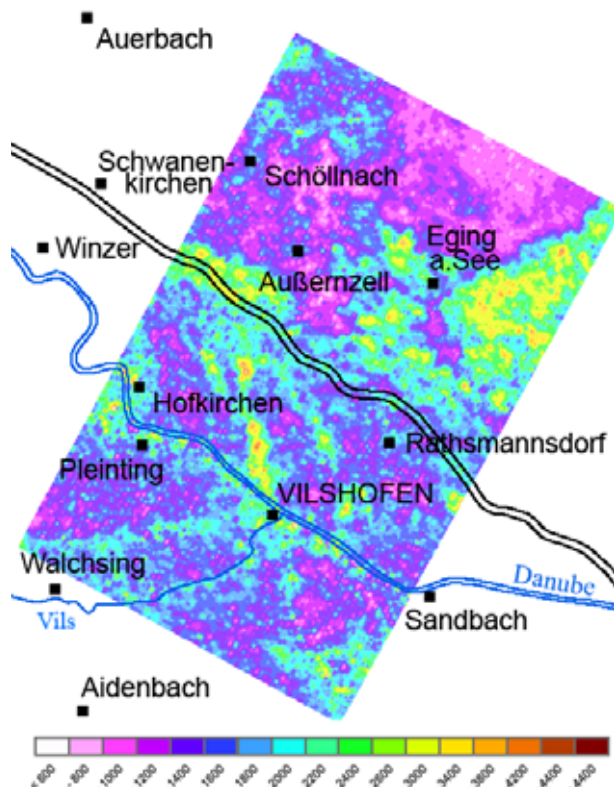
Figure 4 – K/eTh distribution in the airborne survey area. High K/eTh ratios signify a less intense weathering.
