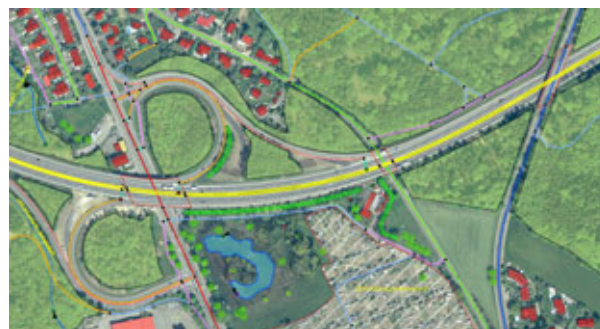
Figure 1: This image is a screenshot from TOPGIS showing TLM data captured on top of an orthophoto. (© 2009 swisstopo)
