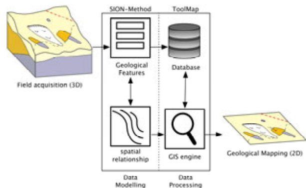
Figure 2 – GIS Framework for digital geological mapping consisting of two components: the SION-Method and TOOLMAP software
