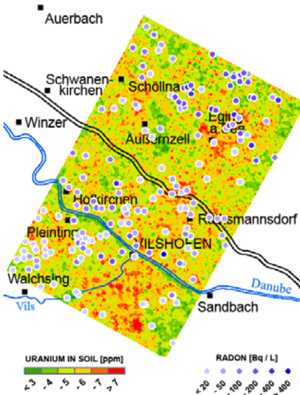
Figure 5 – Uranium eq concentration in near surface horizons as derived from airborne radiometry survey vs. radon activity measurements in groundwater.
