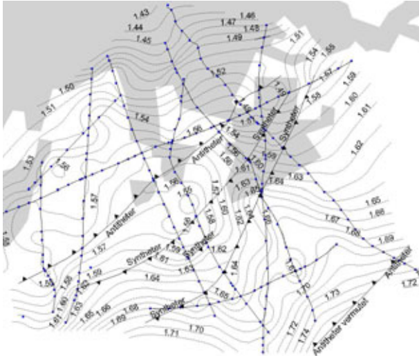
Figure 2 – Detail SE of Munich. Possible interpretation of Lithothamnium-limestone (dots) on seismic lines together with correlation of faults (syn- and antithetic) by 2D-interpretation, still under discussion. Contours are two-way-time (s) for top of Lithothamnium-limestone.
