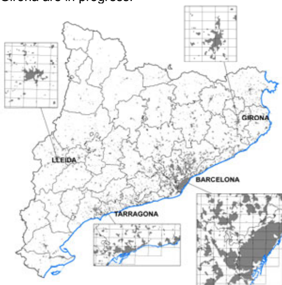
Figure 1 – Map of Catalonia showing the urban areas to be mapped (coloured areas). Boxes depict ongoing urban mapping around province capitals, the grid is the 1:5000 topographic sheet distribution. Solid lines are the county borders.
