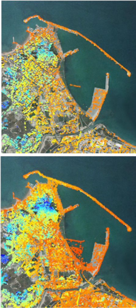
Figure 7. Example of coverage density comparison between Radarsat-1 and new TerraSAR-X data. Each dot corresponds to a PS, hence to a point of measurement.
