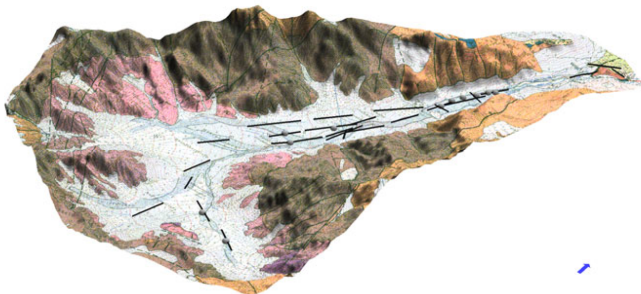
Figure 1 – The Wimbach valley and the location of the seismic profiles (lines) and the geoelectric soundings (spheres).
