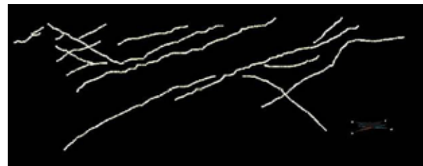
Figure 5 – Joints interpreted from the GPR measurement line seen in Fig. 3. Traces are converted into 3D objects.
