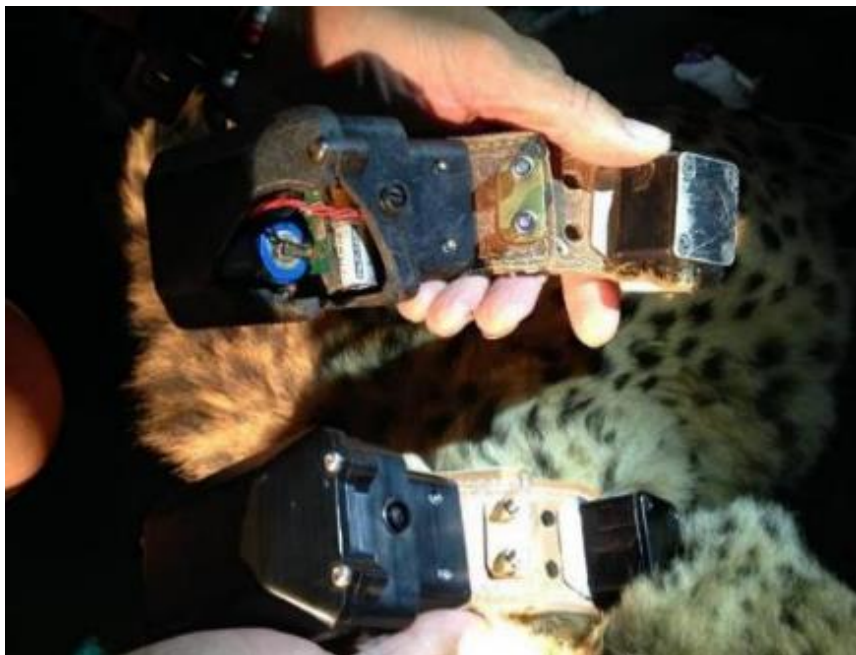
Figure 2: Zinzi's damaged collar (top) compared to the new collar (bottom).
