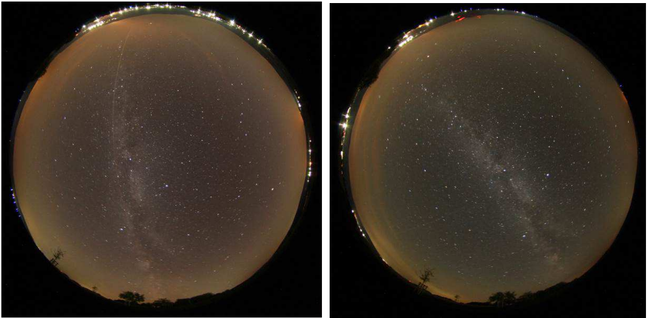
Fig. 9.14: The comparison of the pictures taken at 23:15 (left) and 1:00 (right) showed some reduction of the sky brightness. This might be due to changes in the atmospheric conditions or partly to the partial switch-off in Fladungen. Better atmospheric transmission or switch-offs towards the south (bottom) seems also to reduce the sky brightness.
