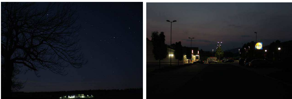
Fig. 7.19: Some positive examples: left: an industrial hall using only full cut-off luminaires that the view towards the stars is not disturbed too much (Frankenheim). Right: a supermarket in the foreground switches off lighting after the end of the business hours, the other one behind uses full cut-off luminaires (Hilders)
