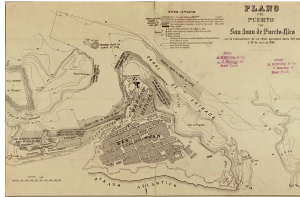
Figure 47. Dredging and landfilled sectors carried out by Spanish government until 1894, San Juan Islet, Puerto Rico. 183
