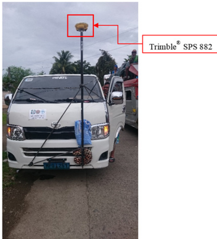
Figure 40. Validation points acquisition survey set-up along the Guinale River Basin
