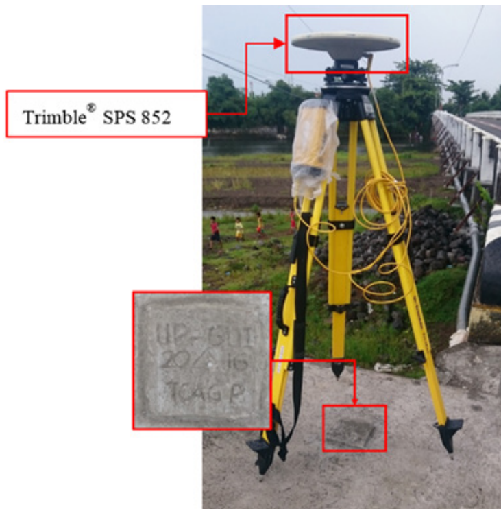
Figure 34. GNSS receiver set-up, Trimble® SPS 852, at UP-GUI, located at the approach of the Imperial Bridge in Barangay Balza, Municipality of Malinao, Albay
