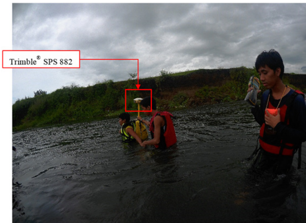
Figure 42. Bathymetric survey using Trimble® SPS 882 in GNSS PPK survey in the Guinale River
