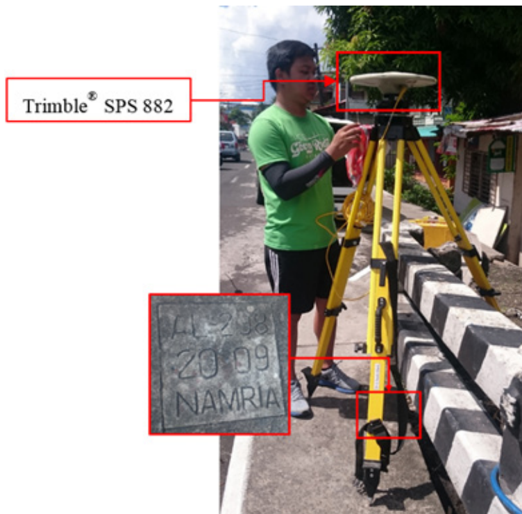
Figure 33. GNSS receiver set-up, Trimble® SPS 882, at AL-298, located at the approach of the Sagpon Bridge in Barangay I-Em's Barrio, Legazpi City, Albay
