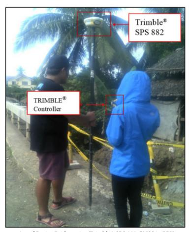
Figure 37. Cross-section of Putiao Bridge using Trimble® SPS 882 GNSS in PPK survey technique
