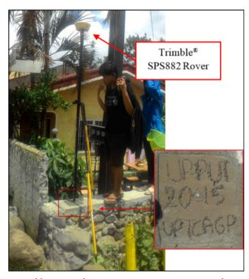
Figure 36. Trimble® SPS882 base set-up at UP-PUT on Putiao Bridge, Lunoy, Pilar
