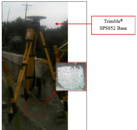
Figure 32. Trimble® SPS852 Base set-up at SR-03 on Putiao Bridge in Lunoy, Pilar
