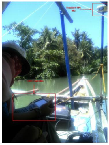
Figure 44. Bathymetric survey using Ohmex™ single beam echo sounder in Putiao River
