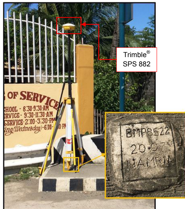
Figure 30. GNSS receiver occupation, Trimble® SPS 882 at PS-522 in Quartel Bridge, Municipality of Sual, Pangasinan
