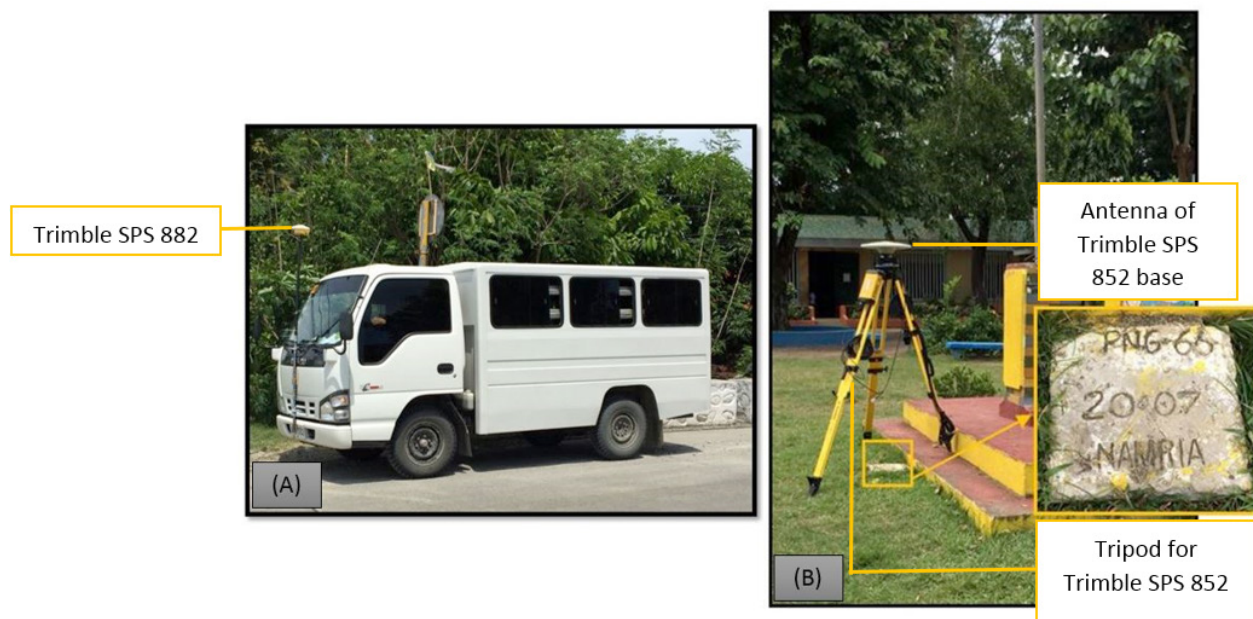
Figure 42. (A) Setup of Trimble® SPS 882 attached to a vehicle and (B) Setting up of GNSS base station at PNG-66
