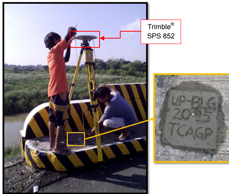
Figure 31. GNSS base receiver setup, Trimble® SPS 852 at UP-BLG in Baloling Bridge, Municipality of Mapandan, Pangasinan
