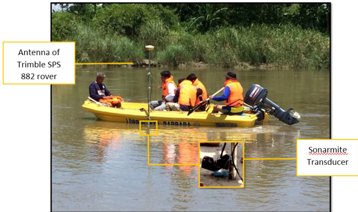
Figure 44. Bathymetric Survey equipment setup on a rescue boat borrowed from PDRRMC of Pangasinan along Sinocalan River
