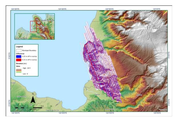
Figure A-8.28. Elevation difference between flight lines
