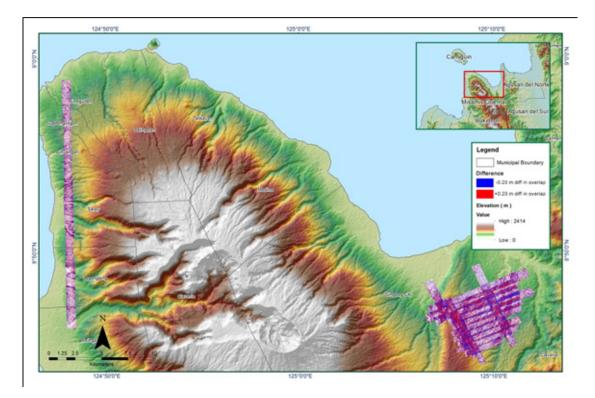
Figure A-8.14. Elevation difference between flight lines
