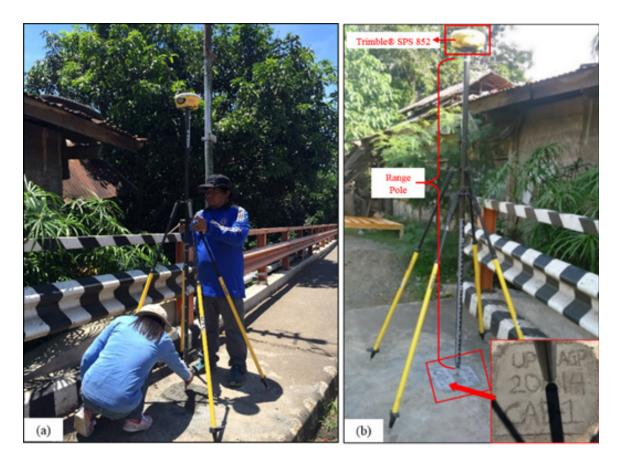
Figure 35. GNSS base occupation, Trimble® SPS 882 at CAB-1 along Iligan-Cagayan de Oro-Butuan Road at the approach of Cabulig Bridge in Brgy. Bobontugan, Municipality of Jasaan, Misamis Oriental.
