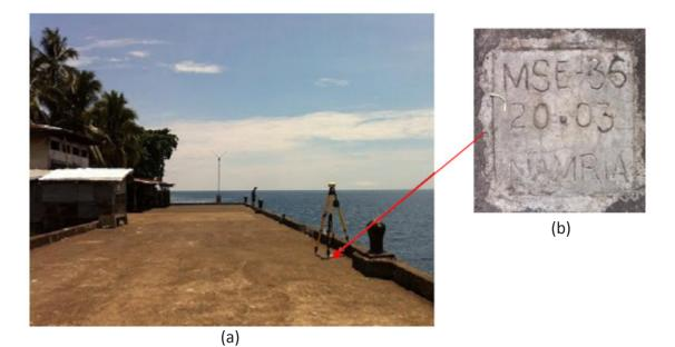
Figure 6. GPS set-up over MSE-36 within Medina municipal port (a) and NAMRIA reference point MSE-32 (b) as recovered by the field team.
