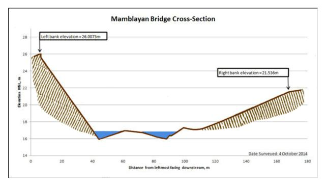
Figure 48. Cross-section plot of Mamblayan Bridge.
