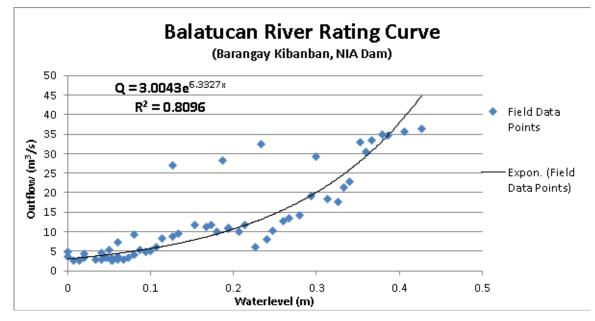
Figure 50. HQ curve of HEC-HMS model.
