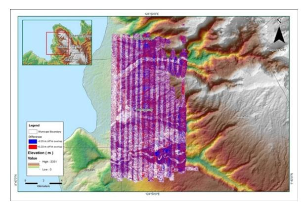
Figure A-8.35. Elevation difference between flight lines
