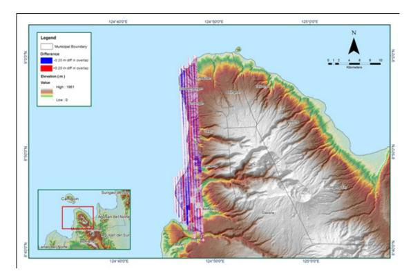
Figure A-8.7. Elevation difference between flight lines
