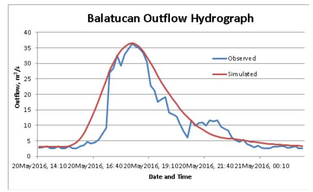
Figure 60. Outflow hydrograph of Balatucan produced by the HEC-HMS model compared with observed outflow.
