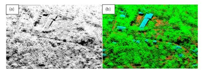
Figure 19. Point cloud before (a) and after (b) classification.
