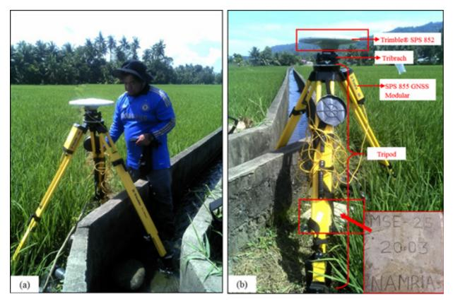
Figure 33. GNSS base receiver set-up, Trimble® SPS 852 at MSE-25 in Brgy. Poblacion 1, Municipality of Villanueva, Misamis Oriental.
