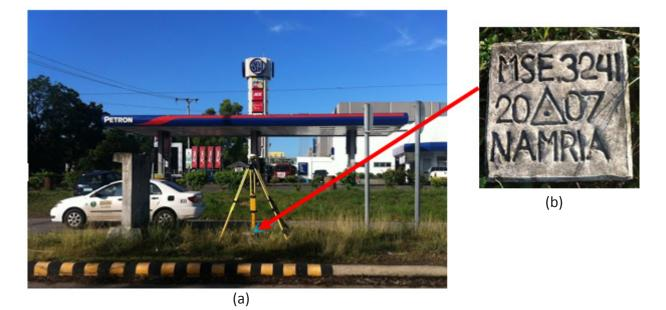
Figure 7. GPS set-up over MSE-3241 on a center island near a gasoline station beside SM Cagayan de Oro (a) and NAMRIA reference point MSE-3241 (b) as recovered by the field team.
