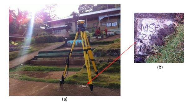
Figure 5. GPS set-up over MSE-32 inside Alicomohan Elementary school, just in front of the school's flag pole, situated at Barangay Alicomohan, Sugbongcogon, Misamis Oriental (a) and NAMRIA reference point MSE-32 (b) as recovered by the field team.
