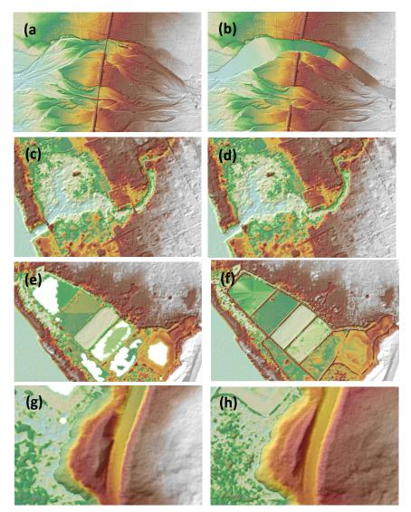
Figure 23. Portions in the DTM of Balatucan Floodplain—bridges before (a), (c) and after (b), (d) manual editing; a paddy field before (e) and after (f) data retrieval; and a misclassified hill before (g) and after (h) data retrieval.
