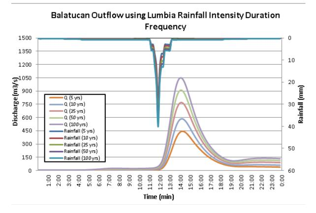
Figure 61. Outflow hydrograph at Balatucan Station generated using Lumbia RIDF simulated in HEC-HMS.
