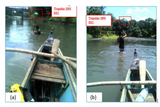
Figure 44. Bathymetric survey: (a) upstream in Barangay Talusan and (b) downstream bathymetry near Barangay Waterfall.
