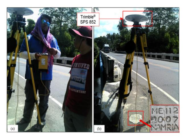
Figure 34. GNSS base receiver setup, Trimble<sup>®</sup> SPS 852 at ME-112 at Musi-Musi Bridge in Brgy. Talusan, Municipality of Balingasag, Misamis Oriental.
