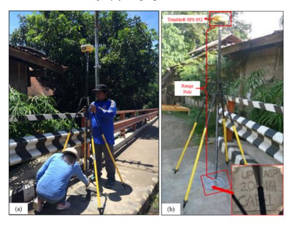
Figure 35. GNSS base occupation, Trimble<sup>®</sup> SPS 882 at CAB-1 along Iligan-Cagayan de Oro-Butuan Road at the approach of Cabulig Bridge in Brgy. Bobontugan, Municipality of Jasaan, Misamis Oriental.
