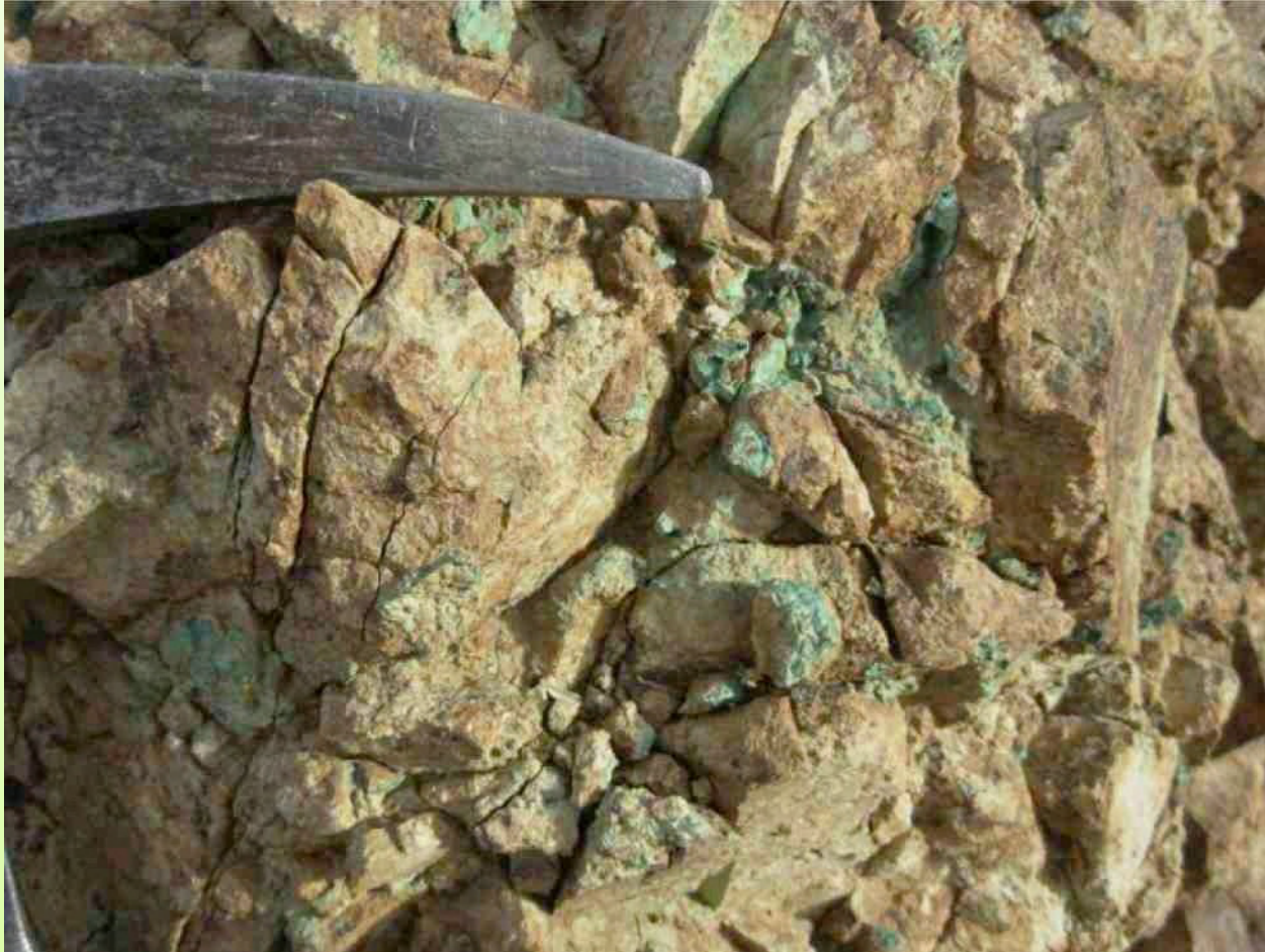
Fracture filling and disseminated Cu-Oxides in altered Granodiorite, Kabul Koh
