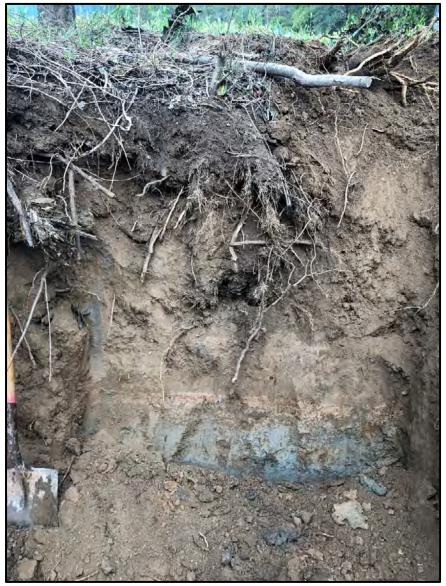
Figure 6.3. Historic alluvium and disturbed soils in UT-1.
