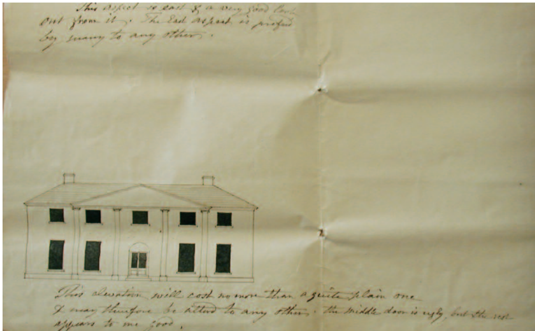
Fig. 13. East elevation of proposed addition to Merton Hall, by Heffer, commissioned by Lord Cadogan, 1804. Norfolk Record Office. Richard Garnier.
