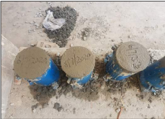
Fig. 03. Concrete cylinders casted 1:2:4 for Mumty slab-GHS Pashtun Garhi, Nowshera
