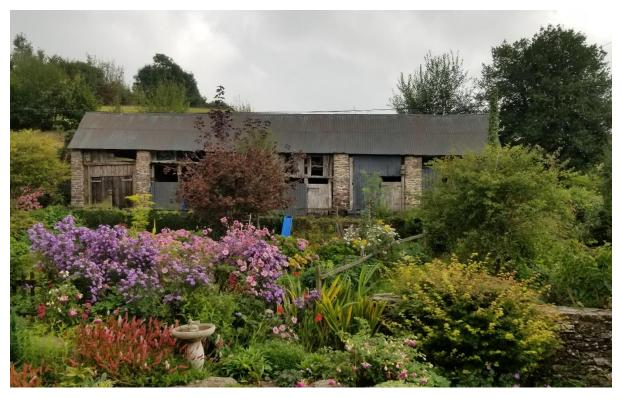
The Linhay. This traditional farm building was in extremely poor condition a few years ago. The land at the rear of the building was pushing it forward and the whole thing was in danger of collapse. Liz's thoughtful and enterprising son made simple but effective repairs by removing the soil from the rear, and then supporting the building by building a breezeblock wall inside to support the roof. A very cost effective and simple repair. Photo by Lizzie Induni
