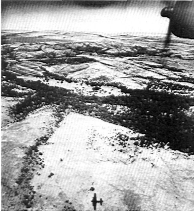
Figure 1—Oblique photograph (focal length 6 inches, tilt 533 mils)
