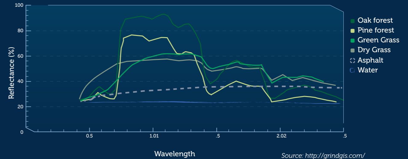
Figure 3. Spectral signatures or responses for different elements of the earth's surface. Each element or land cover has a differential pattern according to the amount of energy it reflects in each wavelength or spectral band, information that is stored in satellite images. Forests present characteristic spectral responses that facilitate their identification (Taken from http://concurso.cnice.mec.es/cnice2006/material121/unidad1/firma_en.htm )
