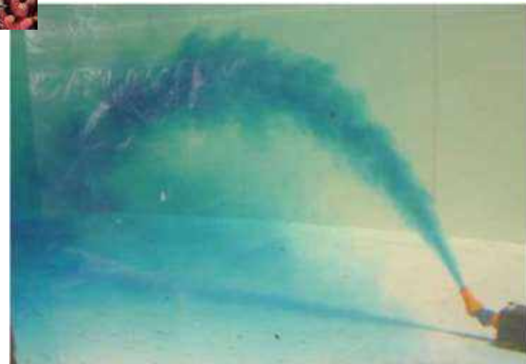
Brine being discharged through a Jet
