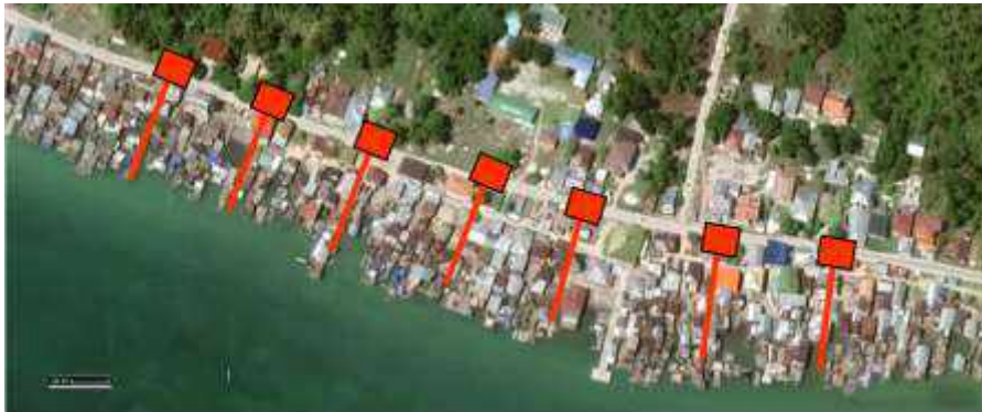
Figure 4.11. Illustrative example of a comb-like network of shared communal sanitation system with a cluster of households along the coastline
