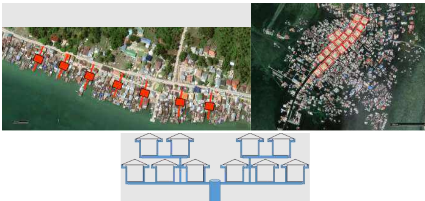
Figure 11. Illustrative example of communal rainwater harvesting clusters
