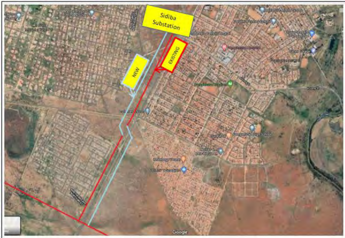
Figure 7.2: Alternative 2 (preferred) for the proposed 132 kV Powerline, near Pampierstad
