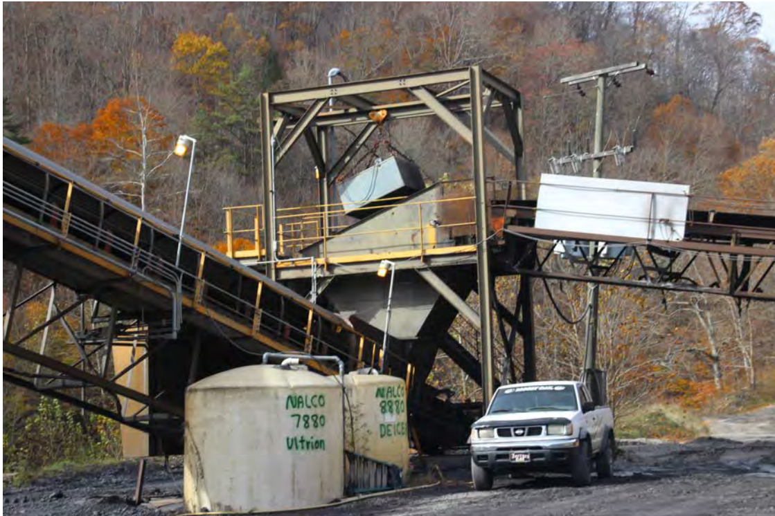
The conveyor belt on the right leads from the mine to this hopper which re-directs the coal into a conveyor belt running at a 90-degree angle from the mine.
