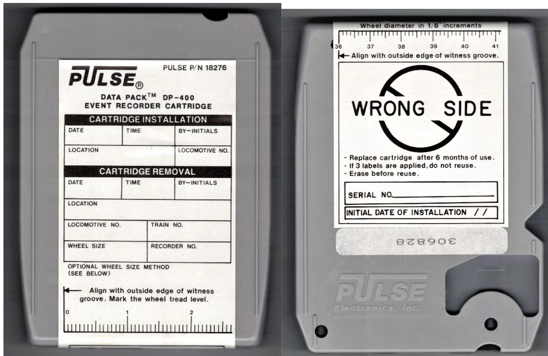
The tape cartridge used in the locomotive event recorder. The tape cartridge is similar to the old 8 track music tape.
