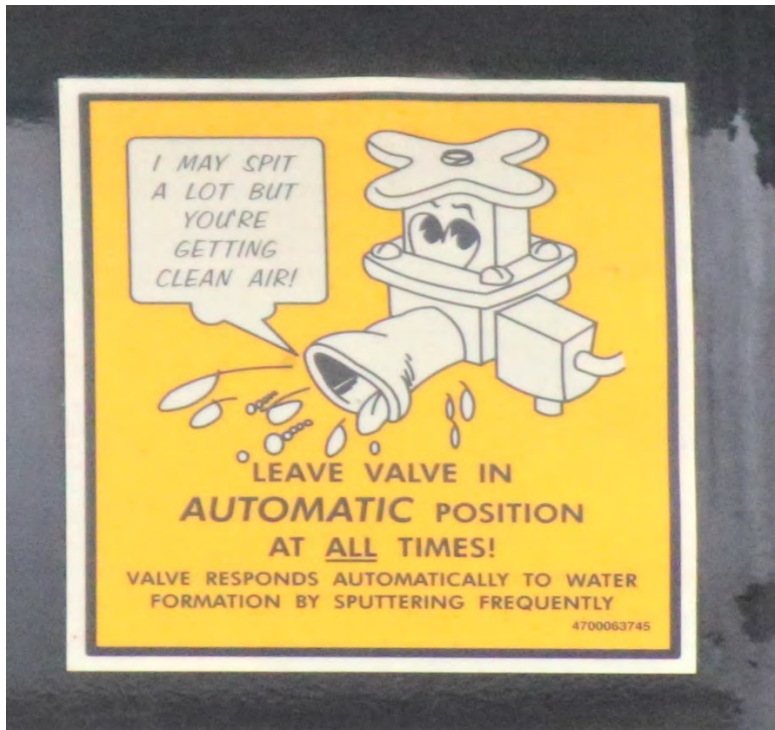
A close-up of the sticker on the air tank telling one and all that it is OK that the air tank randomly squirts moisture into the air as it is just purging its tank of water.
