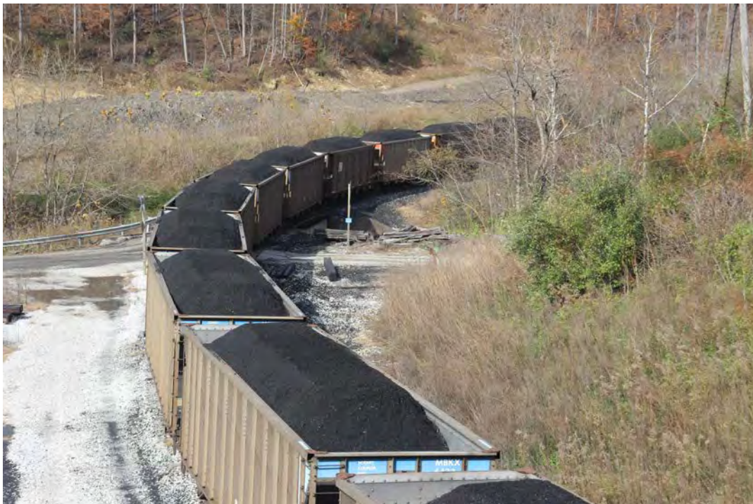
A string of loaded hoppers stretches along the balloon track toward the CSXT track. Normally a 100-car train of 100-ton hoppers can be loaded in 2 to 2.5 hours.
