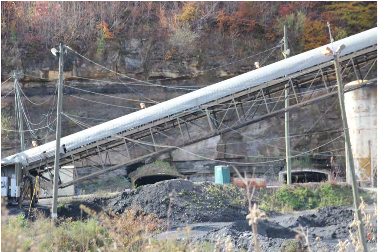
Beyond the conveyor belt are two additional entrances to the mine. These were not being used as the area was mined out. Only the coal pillars remained to be harvested.
