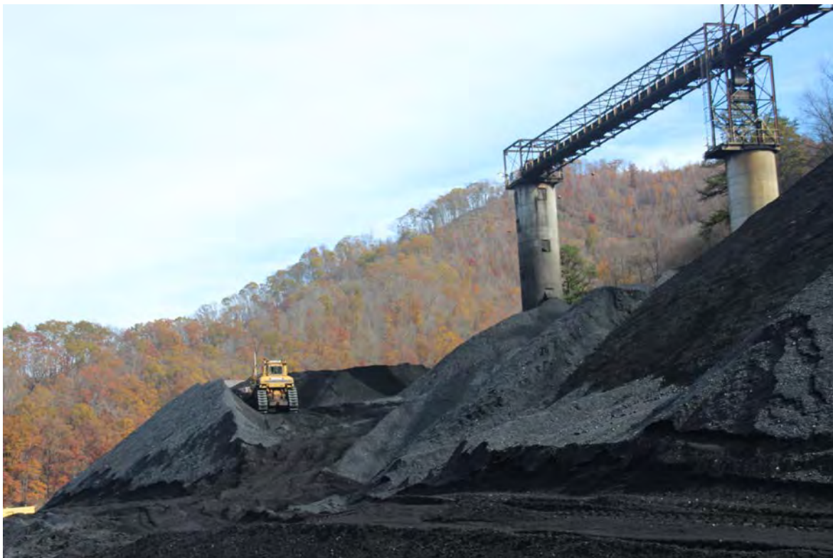
Above and below is the coal storage area. Underground augers carry the coal from here to a conveyor belt that leads to the train flood loading tippie. Note in the photo below the D9 bulldozer working the coal pile. Coal is dumped into the top of the cylinders and falls out to the storage area through window cut in the cylinder walls.
