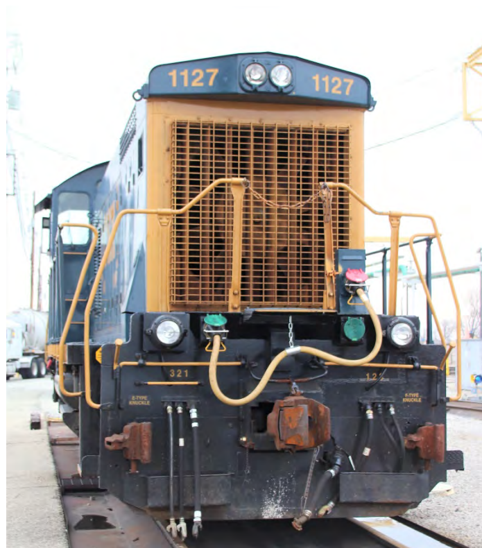
A view of the front of CSXT 1127 showing the radiator vent and her MU cable and replacement knuckles
