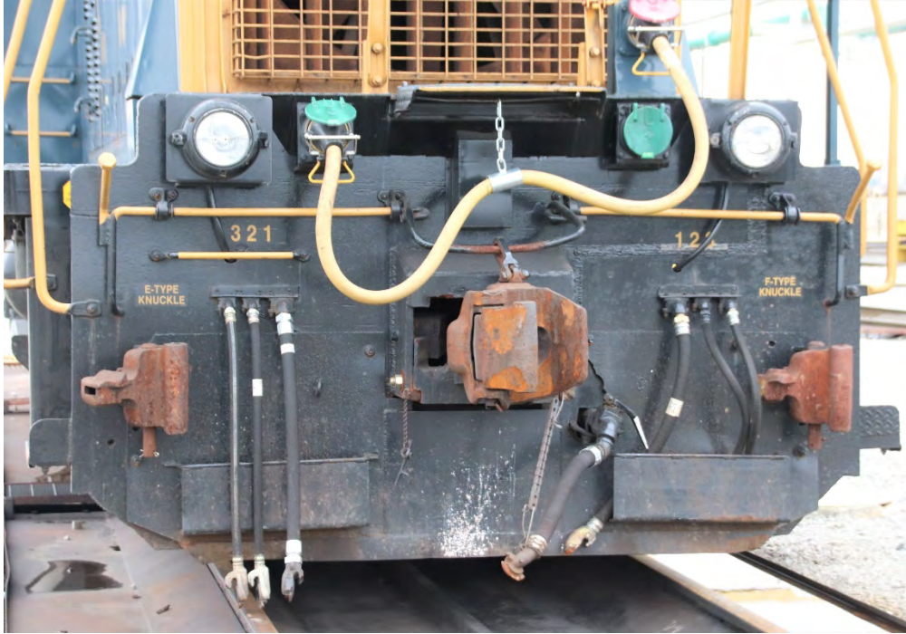
A close-up of CSXT 1127 snow plow. On the right she carries a spare F knuckle and on the left a spare E Type Knuckle
