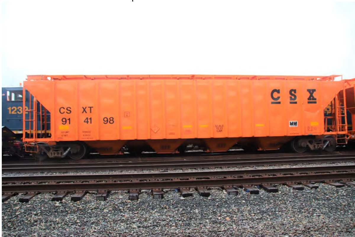
Scale Test Car CSXT 914198 is a converted cover hopper.
