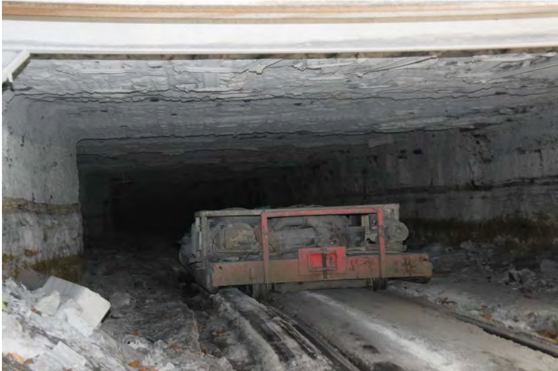
The mine cart that delivers the miners to the coal face. The tunnel is 40-inches high and ten-feet wide.
