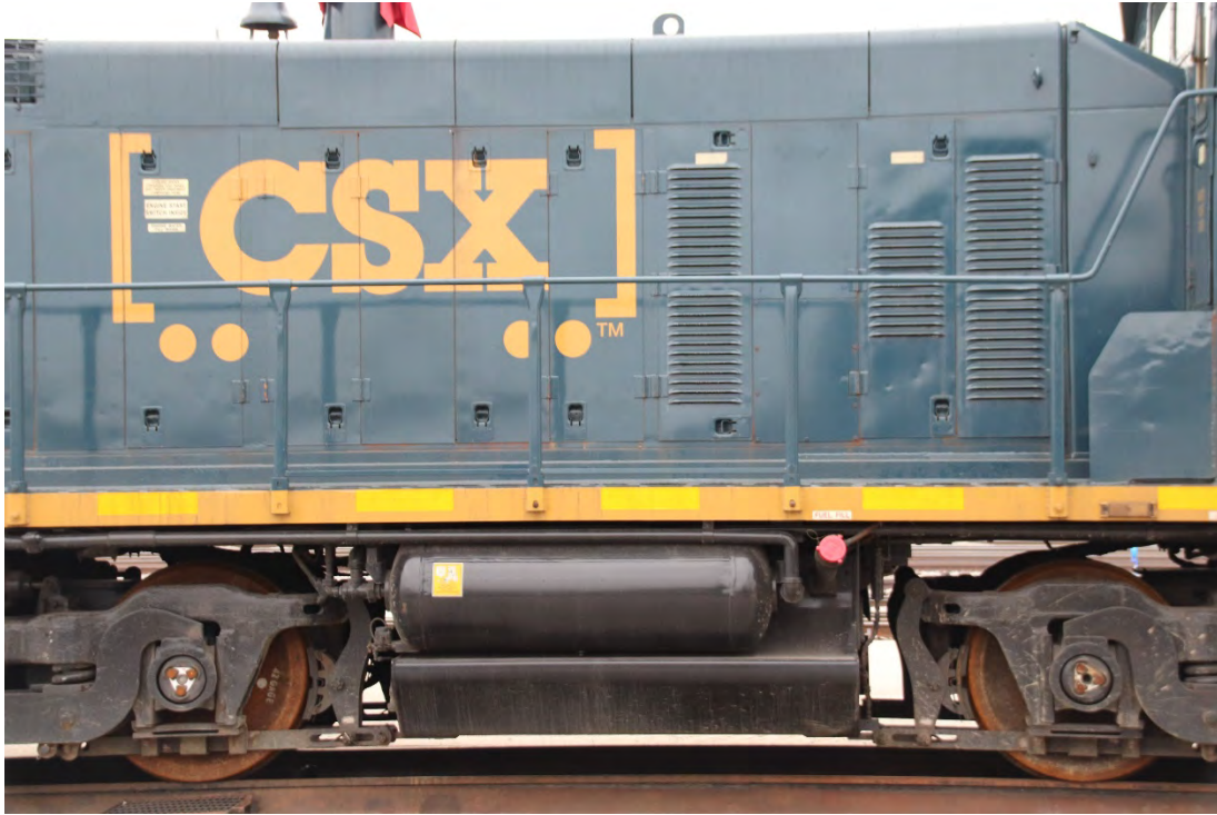
A view of the right-side fuel tank and air reservoir
