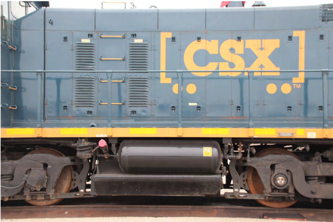
A view of the left side fuel tank with the air reservoir on top of the fuel tank
