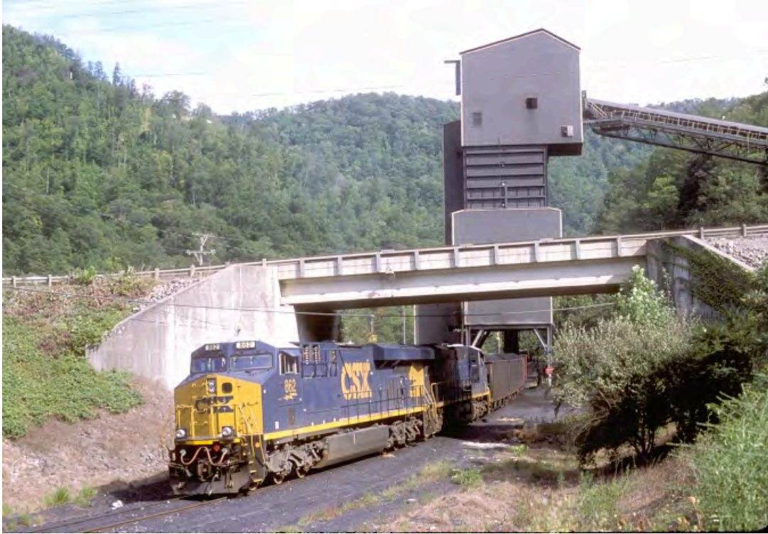
CSXT 862, a GE CW46AC/H, and a sister locomotive lead a unit train through the flood loader. The bridge carries the site's road over the track and up the hollow to the wash plant. (Blue Diamond Mine)
