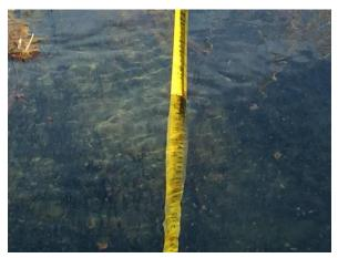
**Photo #4** Measuring the depth, approximately 16 feet below grade surface, of borehole (March 2016).
