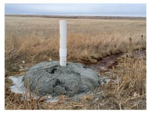
**Photo #7** View (looking southeast) of grouted and cased borehole (March 2016).
