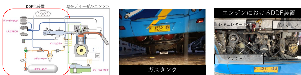
Figure 1-1 DDF system and a case of installation in a public bus in Semarang
